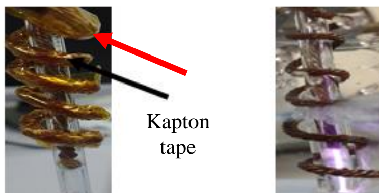
Figure 2 Ground electrode; 2(i) insulated ground electrode, 2(ii) non-insulated ground electrode.
