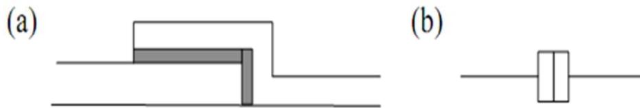
Fig. 1: (a) an overlap junction with an oxide layer (b) schematic diagram for a tunnel junction.
