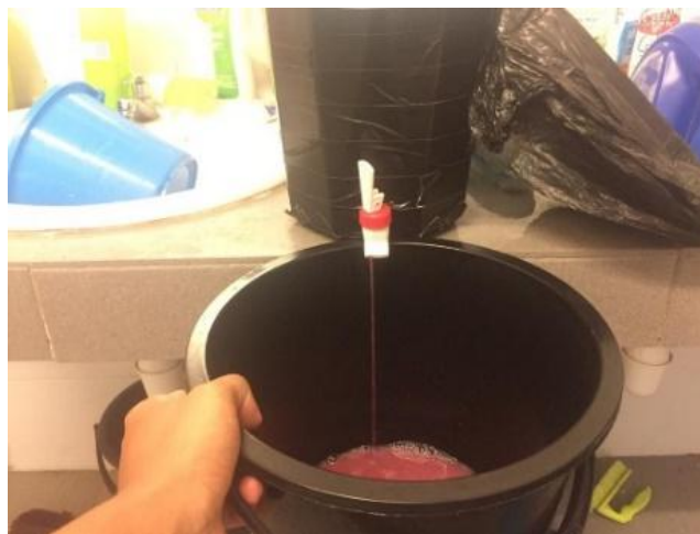
Figure 3. Drawing out liquid to ensure the occurrence of aerobic degradation.
