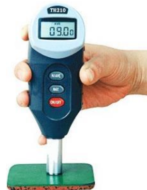
Figure 1 Hardness test (TH210 Shore Durometer)
