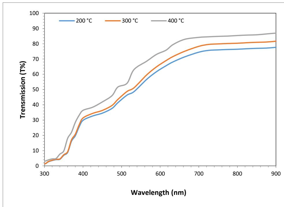
**Figure 2.** Transparency of CdO at various substrate temperatures.
