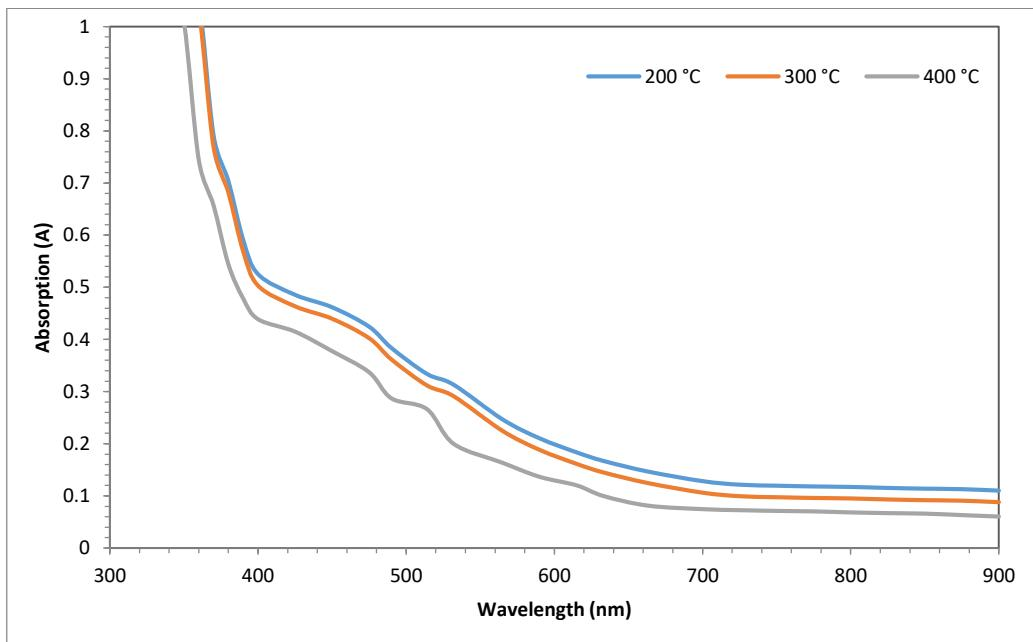
**Figure 3.** Optical absorption of CdO at various substrate temperatures.
