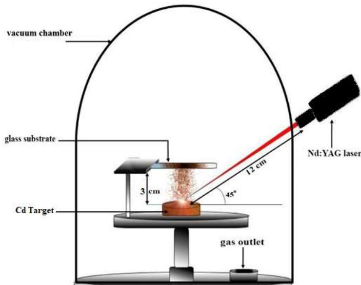
**Figure 1.** System diagram for pulsed laser deposition system.
