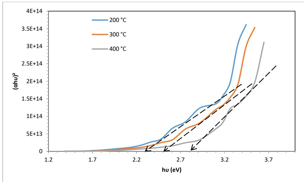
**Figure 4.** Optical band gaps of CdO at various substrate temperatures.
