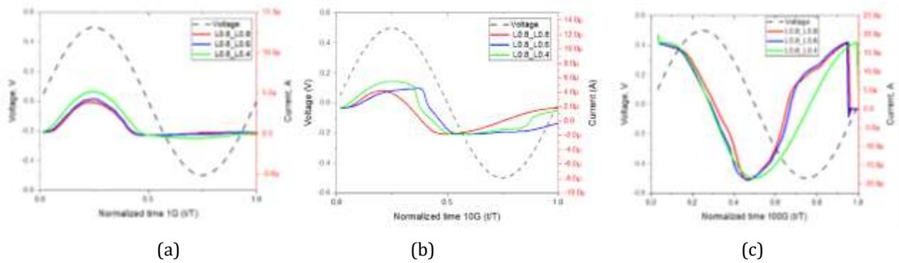
**Figure 6.** AC transient analysis of parallel SSDs at frequencies of (a) 1 GHz, (b) 10 GHz, and (c) 100 GHz for different pair channel lengths.
