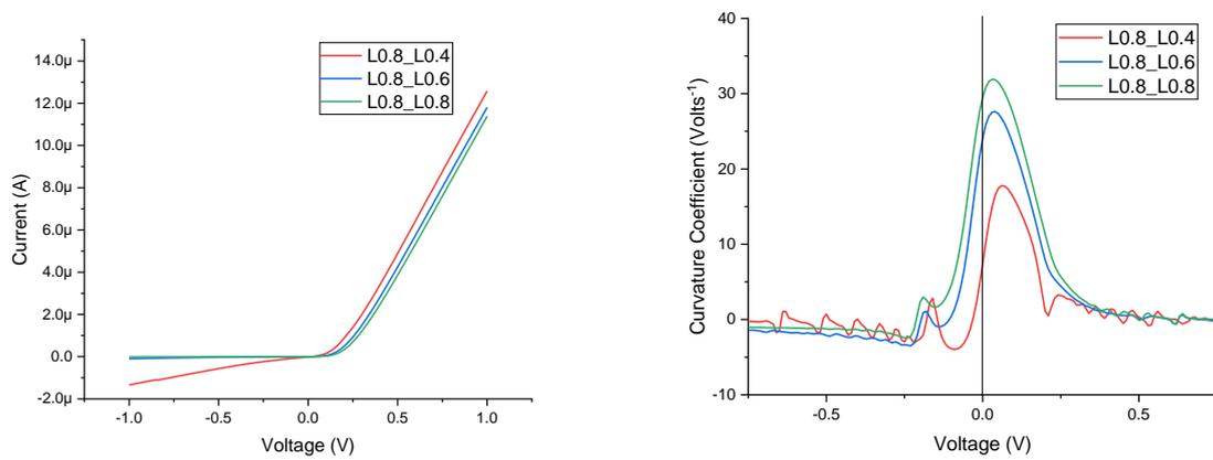
**Figure 4.** (a) I-V behavior of parallel InGaAs SSDs and (b) Rectification performance measured by the device curvature coefficient in relation to the applied voltage for different pair channel lengths.
