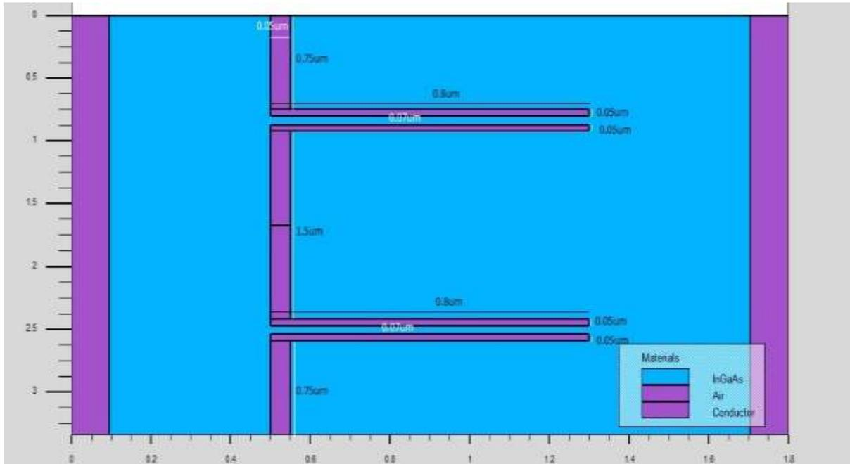
**Figure 2.** Two InGaAs-based SSDs connected in parallel dimensions.
