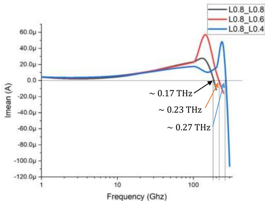
**Figure 7.** Mean output current,  $I_{mean}$ , and the cut-off frequency,  $f_c$ , results for various pair channel lengths.
