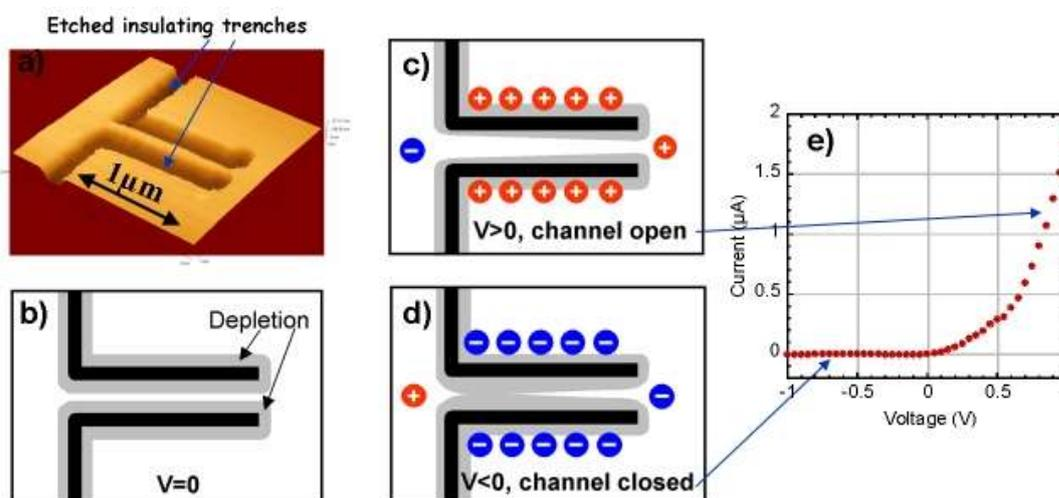
**Figure 1.** (a) An AFM image of a single SSD. (b) The grey area (native depletion region) was formed using etched interfaces. (c) Applying positive voltage will open the device channel. (d) Applying negative voltage will close the device channel. (e) Single SSD I-V characteristics [6].
