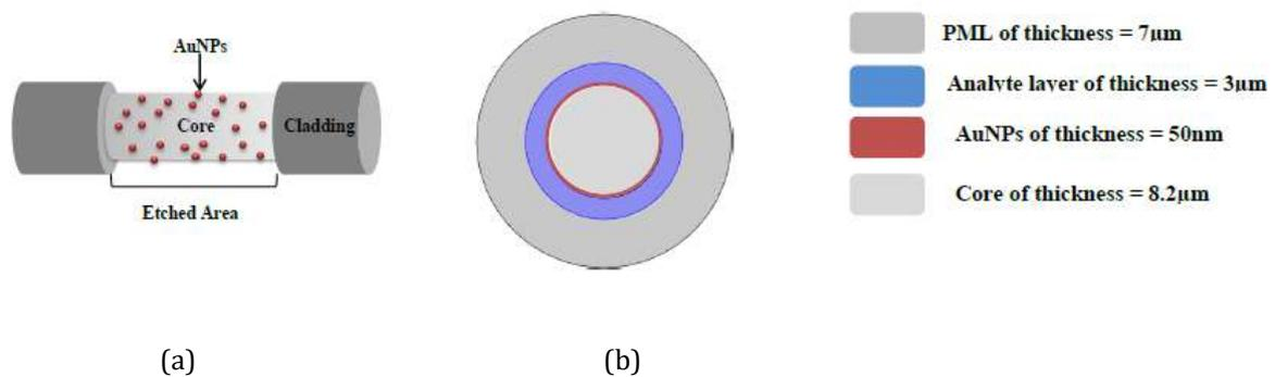
**Figure 1.** Presents a) the geometry of etched fiber, and b) Cross section of the proposed sensor.
