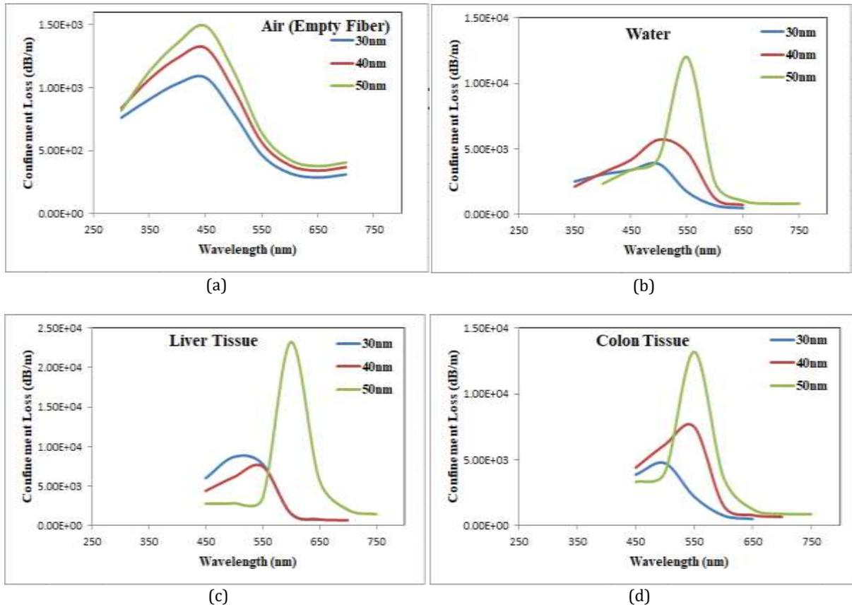
**Figure 2.** Presents the confinement loss (dB/m) of (a) Air (empty fiber), (b) water, (c) Liver tissue, and (d) Colon tissue, at AuNPs thickness of 30, 40, 50nm.
