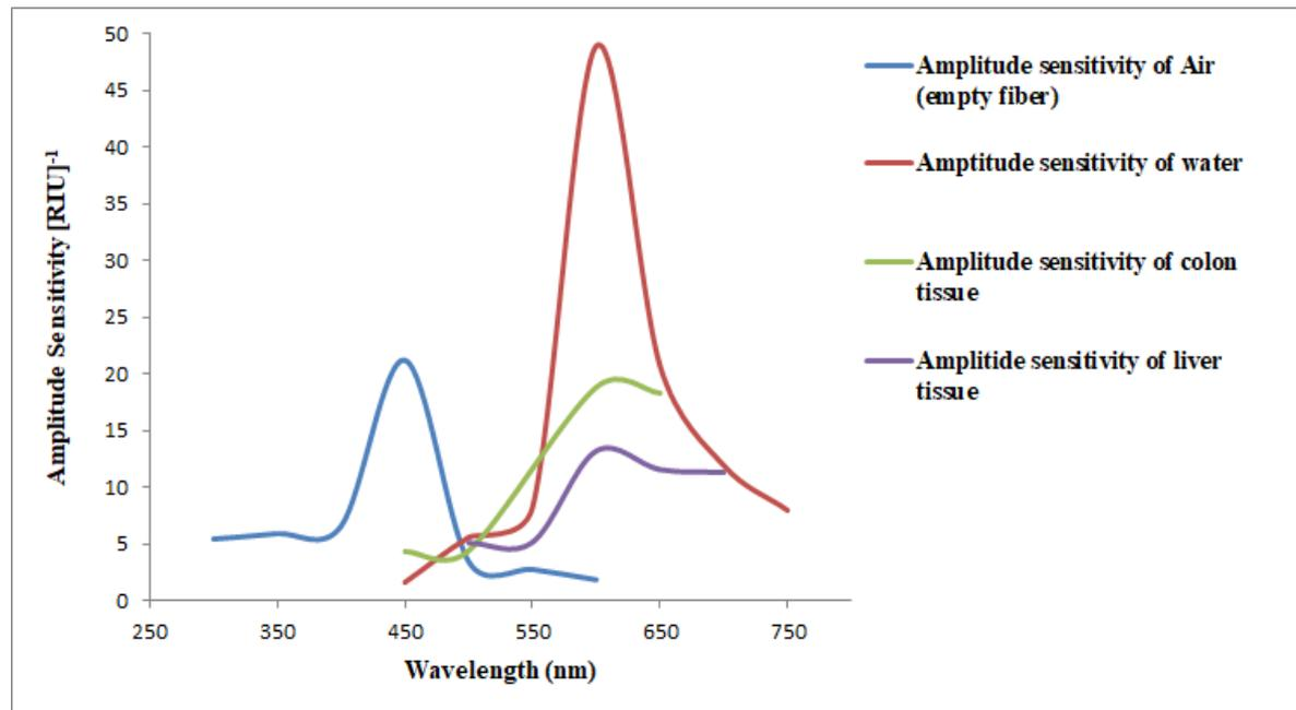
**Figure 5.** Presents the amplitude sensitivity in [RIU]<sup>-1</sup> for air, water, liver tissue, and colon tissue.
