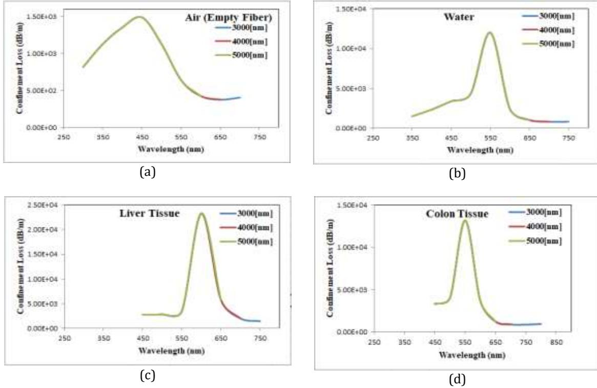
**Figure 4.** Presents the confinement loss (dB/m) of a) Air (empty fiber), b) Water, c) Liver tissue, and d) Colon tissue, at analyte layer thickness of 3000, 4000, and 5000nm.
