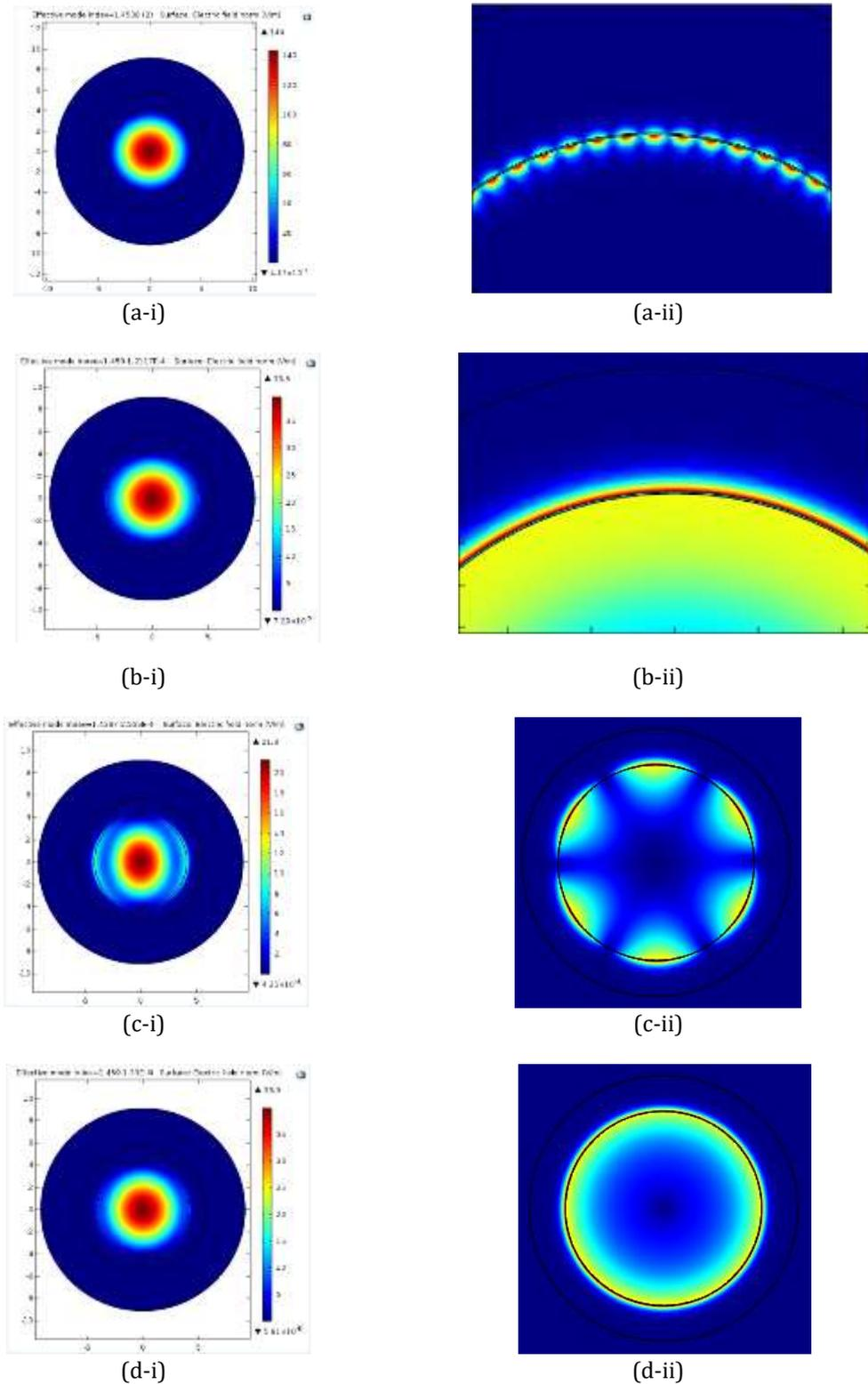
**Figure 3.** Presents shows the electric field dispersion spectrum of a-i) the fundamental core mode, and a-ii) The SPR mode, at 400nm for air (empty fiber), b-i) the fundamental core mode, and b-ii) The SPR mode, at 550nm for water, c-i) the fundamental core mode, and c-ii) The SPR mode, at 600nm for liver tissue, and of d-i) the fundamental core mode, and d-ii) The SPR mode, at 550nm for colon tissue.
