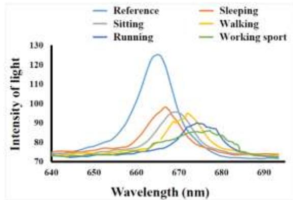
**Figure 9.** Transmission spectra of 5 cm coreless fiber interferometer coated with gold & graphene with different breathing cases.
