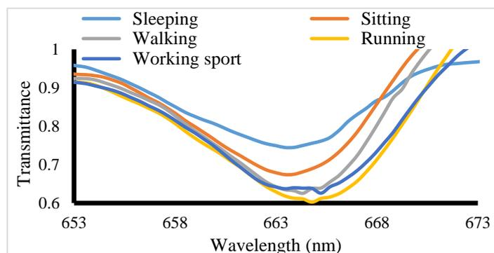
**Figure 10.** Transmittance spectra of 5 cm coreless fiber interferometer coated with gold & graphene with different breathing cases.
