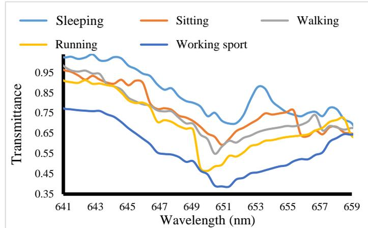
**Figure 5.** Transmittance spectra of 5 cm coreless fiber interferometer coated with gold nanoparticles with different breathing cases.
