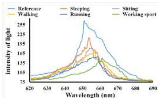
**Figure 4.** Transmission spectra of 5 cm coreless fiber interferometer coated with nanogold particles with different breathing cases.
