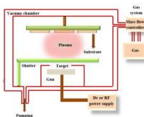
**Figure 1.** Schematic diagram of a mechanism of magnetron sputter coating machine.
