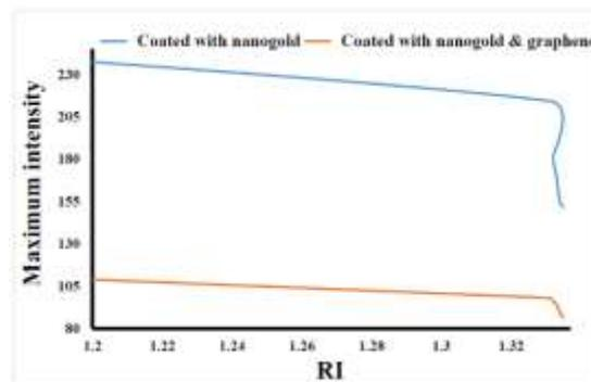
**Figure 13.** Maximum intensity vs. refractive index of sensor coated with nanogold and nanogold & graphene.
