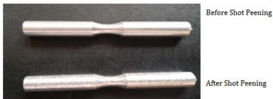
Figure 6. Specimens before and after shot peening.
