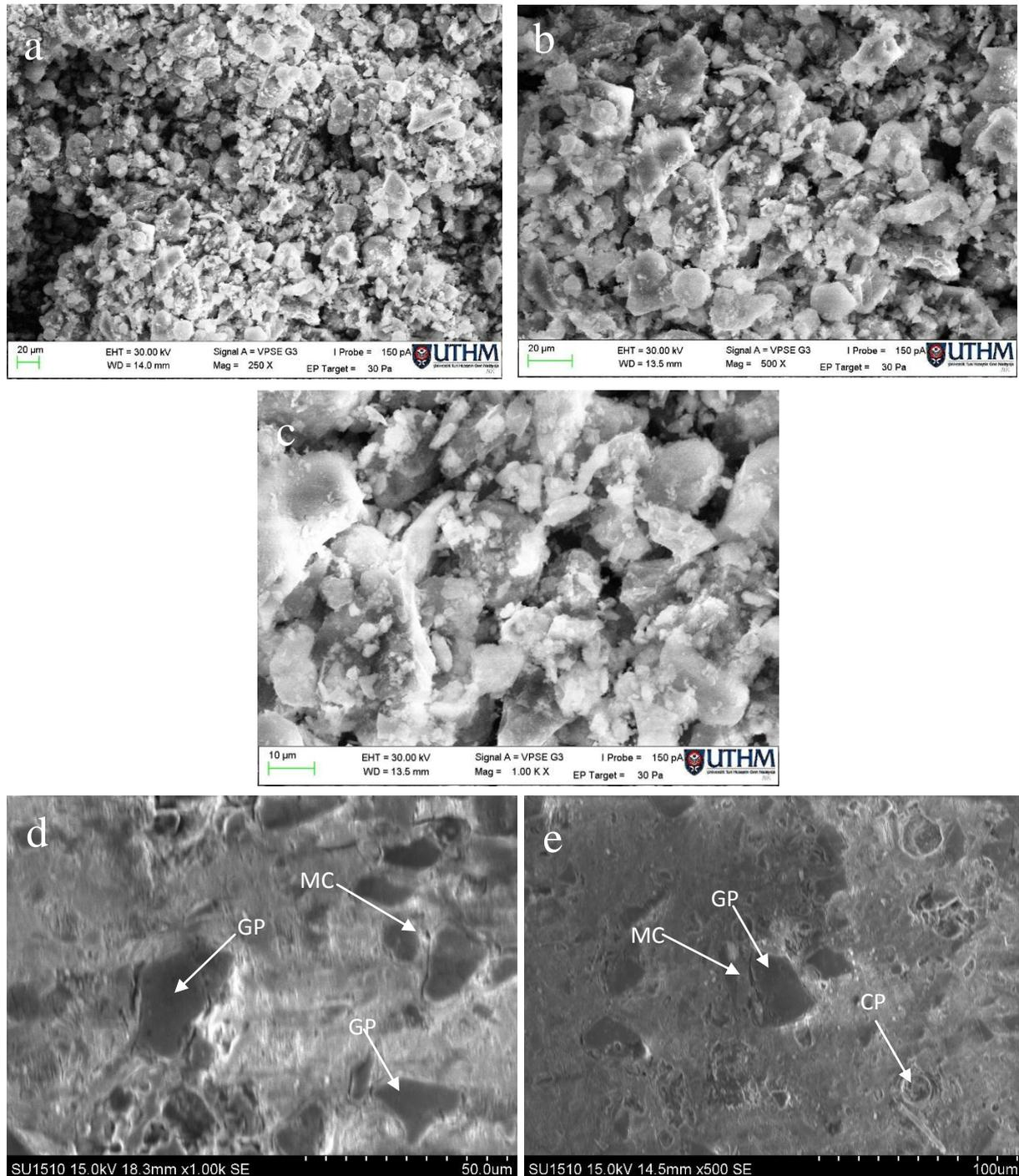
Figure 1. SEM of POFA powder (a,b and c) and porcelain without addition of ferum  $Fe_2O_3$  (d) and after addition (e). [MC = micro crack, CP = closed porosity, GP = Glassy phase]
