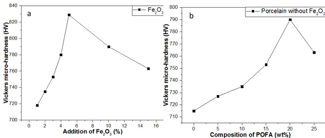
Figure 5. Vickers micro hardness of Porcelain made with and without addition of  $\text{Fe}_2\text{O}_3$ .
