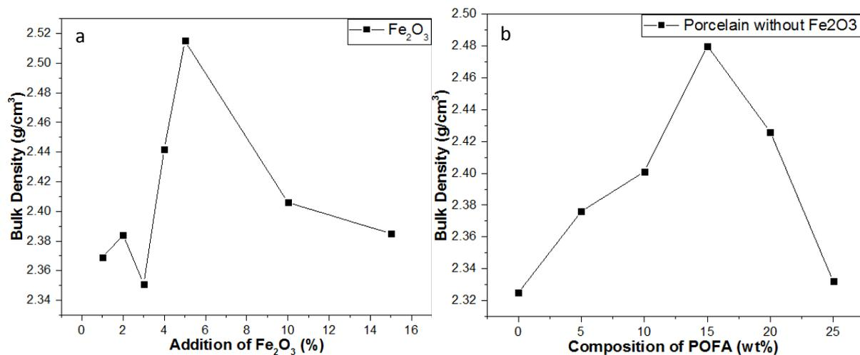
Figure 4. Bulk density of porcelain with and without addition of  $\text{Fe}_2\text{O}_3$
