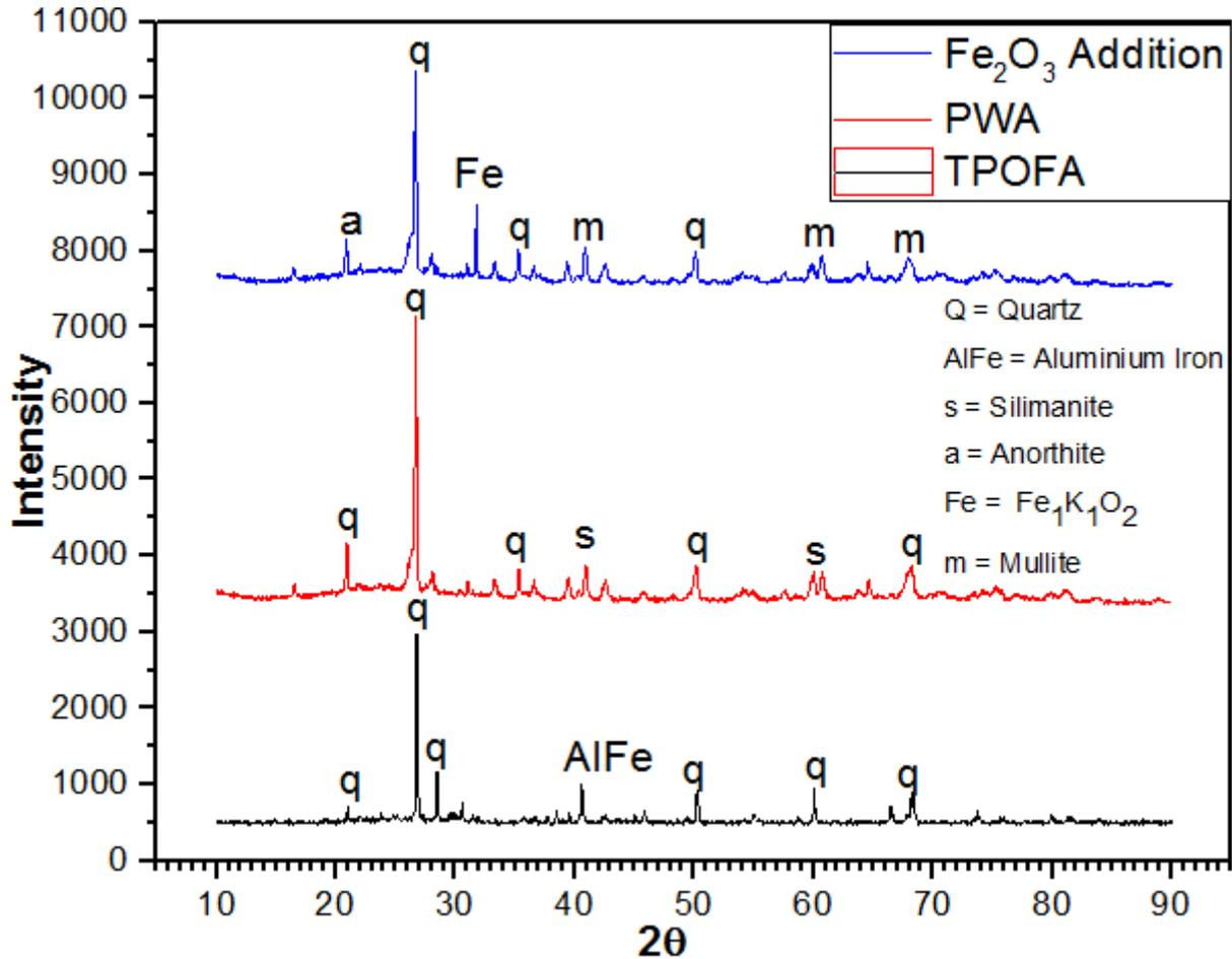
Figure 2. XRD pattern of treated POFA (TPOFA), porcelain without addition of  $\text{Fe}_2\text{O}_3$  (PWA) and porcelain with addition of  $\text{Fe}_2\text{O}_3$ .
