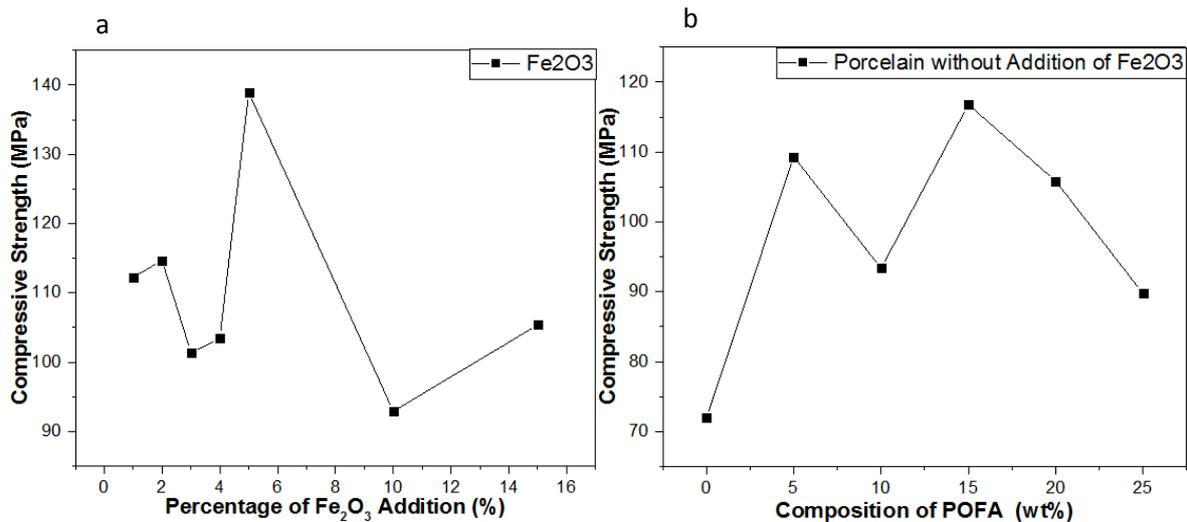
Figure 3. Compressive strength of porcelain with and without addition of  $\text{Fe}_2\text{O}_3$
