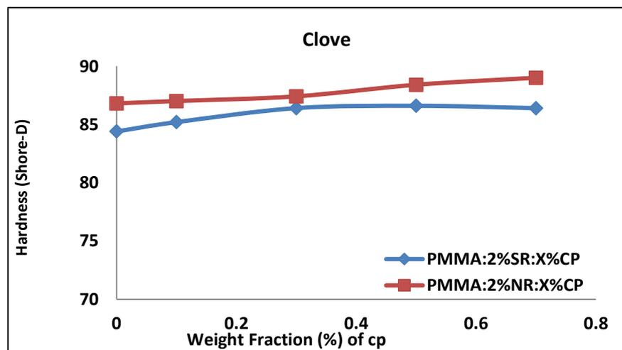
**Figure 12.** Hardness for PMMA bio composite specimens as a function of weight fraction content for (CP powder) in composites.
