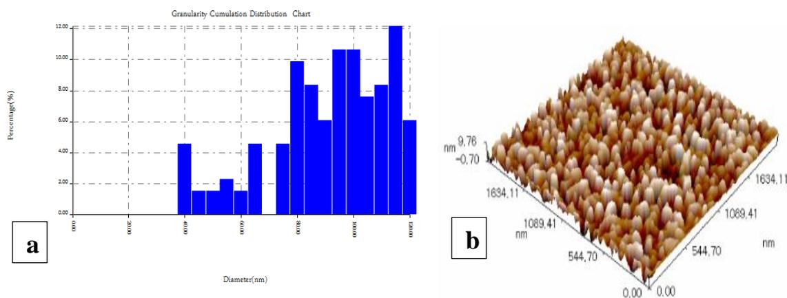
**Figure 2.** AFM test of clove powder nanoparticles with average diameter 75.18 nm, where a: Granularity accumulation distribution chart of clove powder and b: Three-dimensional (XYZ) AFM pictures for clove powder
