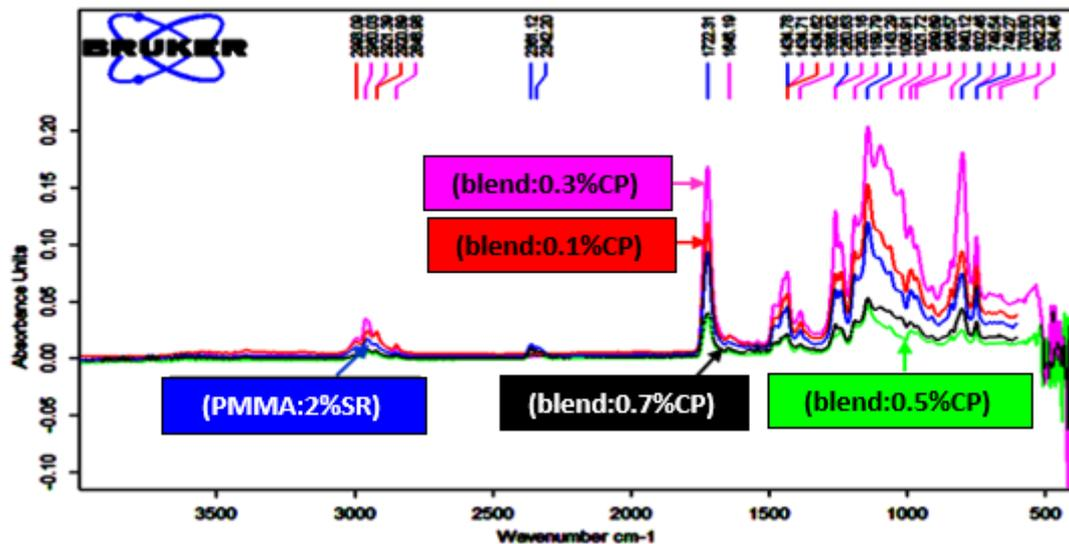
**Figure 6.** FTIR spectra for polymer blend (PMMA: 2%SR) and polymer blend composites ((PMMA: 2%SR): X% CP) as a function of Nano Clove powder content in composite.
