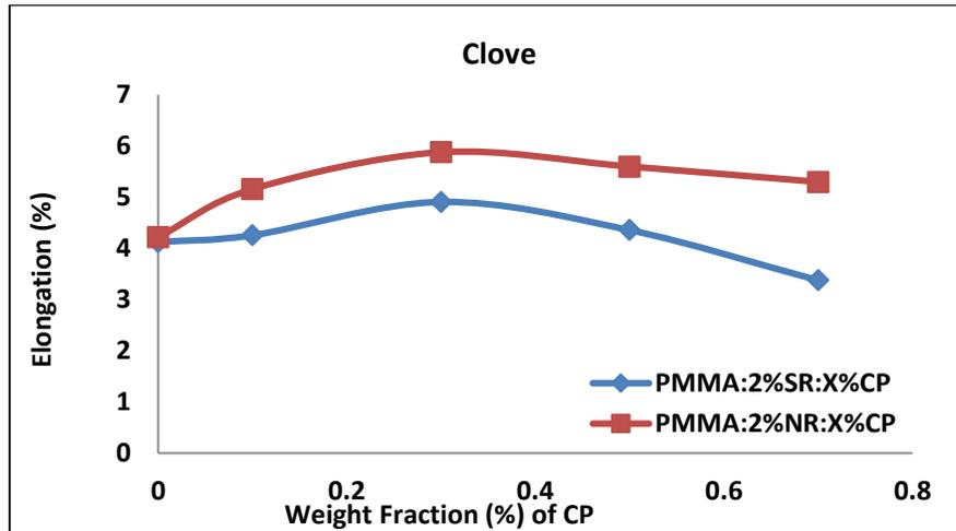
**Figure 11.** The percentage of elongation at break for PMMA bio composite specimens as a function of weight fraction content for (CP powder) in composites.
