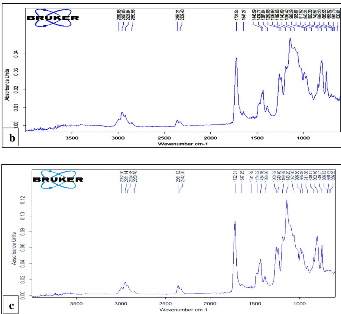
**Figure 3.** The Infrared Spectrum for a: Neat PMMA (heat curing), b: Polymer blend (PMMA: 2% NR) and c: Polymer blend (PMMA: 2% SR).
