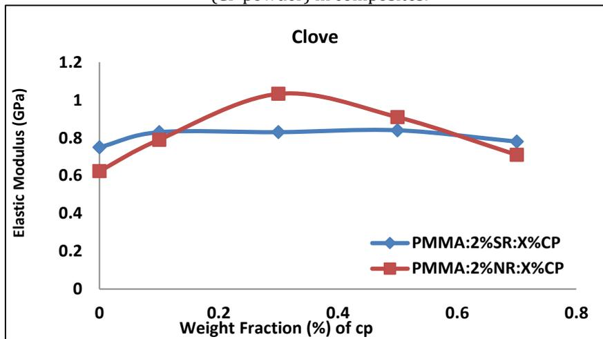
**Figure 10.** Elastic modules for PMMA bio composite specimens as a function of weight fraction content for (CP powder) in composites.
