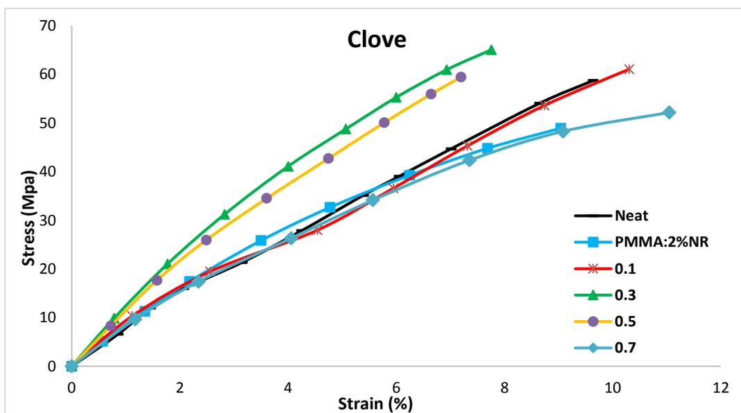
**Figure 7.** Stress-strain curve for PMMA bio composite specimens (PMMA:2%NR:X%CP) as a function of weight fraction content for (CP powder) in composites.
