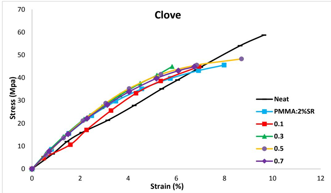
**Figure 8.** Stress-strain curve for PMMA bio composite specimens (PMMA:2%SR:X%CP) as a function of weight fraction content for (CP powder) in composites.
