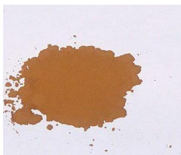
**Figure 1.** Reinforcement material: (Clove powder) having nanoparticles size (75.18 nm)
