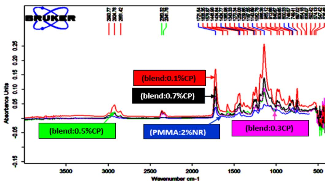
**Figure 5.** FTIR spectra for polymer blend (PMMA: 2%NR) and polymer blend composites ((PMMA: 2%NR): X% CP) as a function of Nano Clove powder content in composite.
