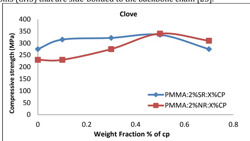
**Figure 13.** Compression strength for PMMA bio composite specimens as a function of weight fraction content for (CP powder) in composites.
