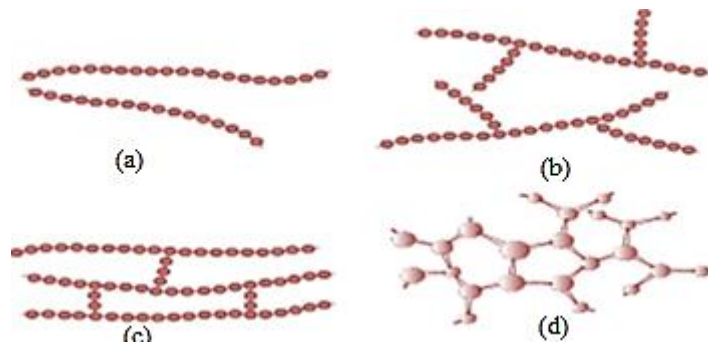
Figure 1 . Graph representations of (a) linear, (b) branched, (c) cross-linked, and (d) network (3-dimensional)molecular structures. Circles designate individual repeated units [7].
