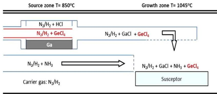
Figure 1. Schematic diagram of horizontal HVPE reactor [39].
