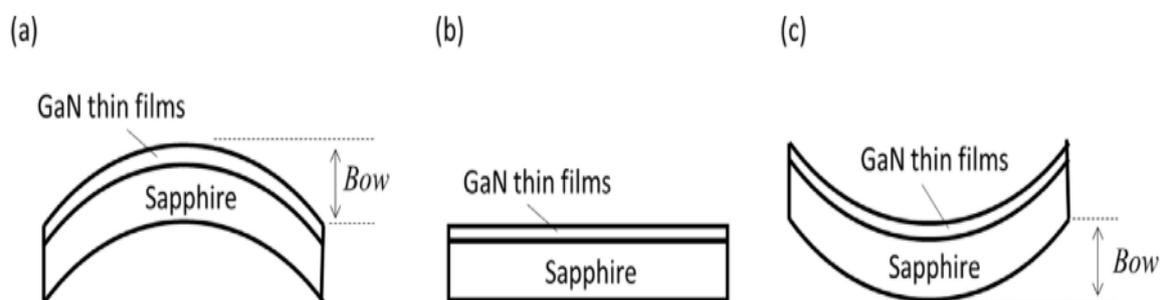
**Figure 8.** Bowing characteristics of (a) convex, (b) flat and (c) concave shapes [67].
