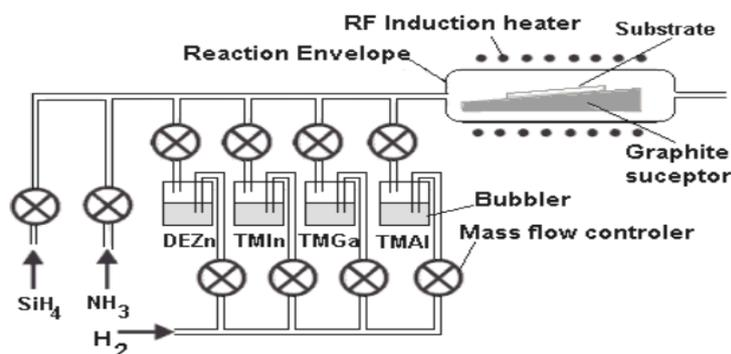
Figure 2. Schematic diagram of MOCVD technique [33].
