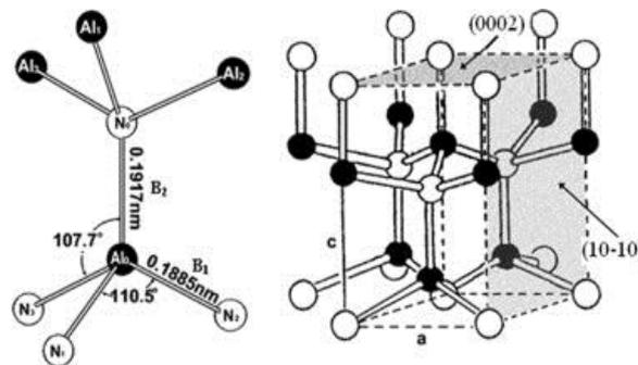
**Figure 4.** Schematic diagram of wurtzite AlN crystal structure [58].
