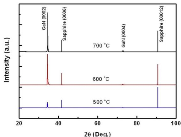
Figure 10. HRXRD  $2\theta/\omega$  spectra of GaN layers [50].
