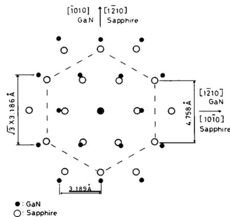
**Figure 5.** Crystal structure of GaN and sapphire [31].
