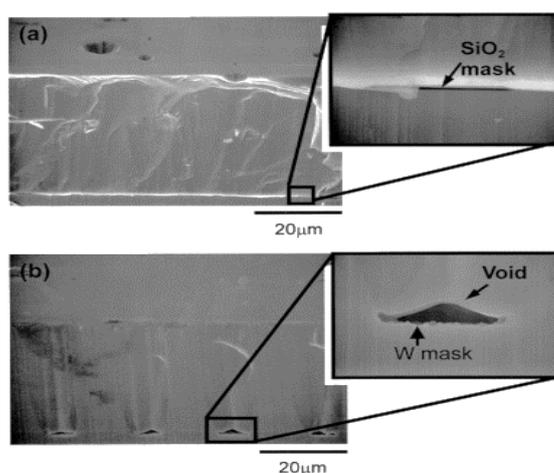
**Figure 6.** SEM cross-section images of GaN on (a) SiO<sub>2</sub> and (b) stripe tungsten mask [59].
