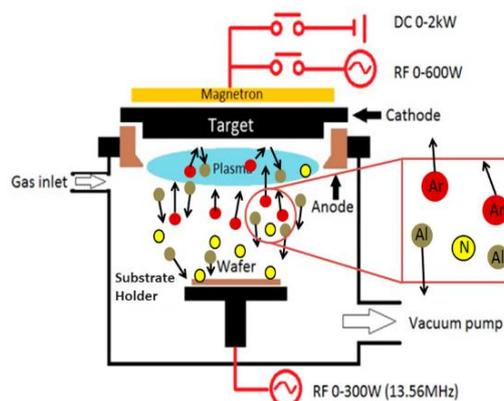
**Figure 18.** Schematic diagram of sputtering process [94].
