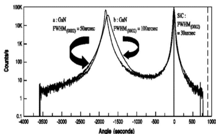
**Figure 12.** X-ray rocking curve of a GaN/SiC heterostructure on (a) treated SiC and (b) pure SiC.
