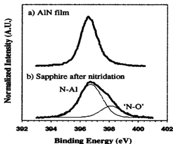
**Figure 7.** XPS peaks of (a) standard AlN film and (b) sapphire substrate after nitridation [64].
