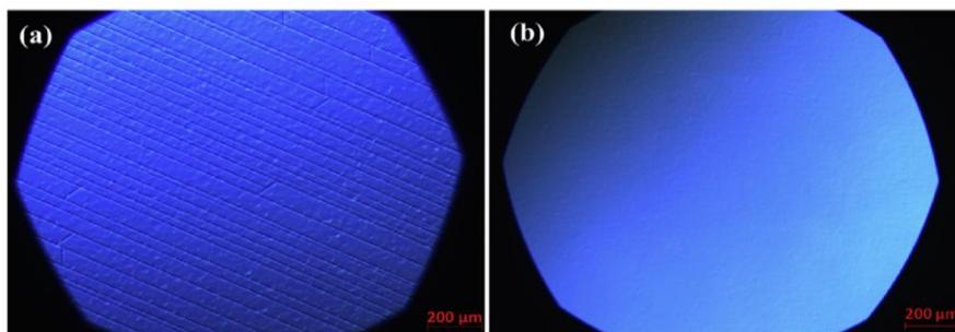
**Figure 16.** GaN surface layer (a) without new cleaning process and (b) with new cleaning process[91].
