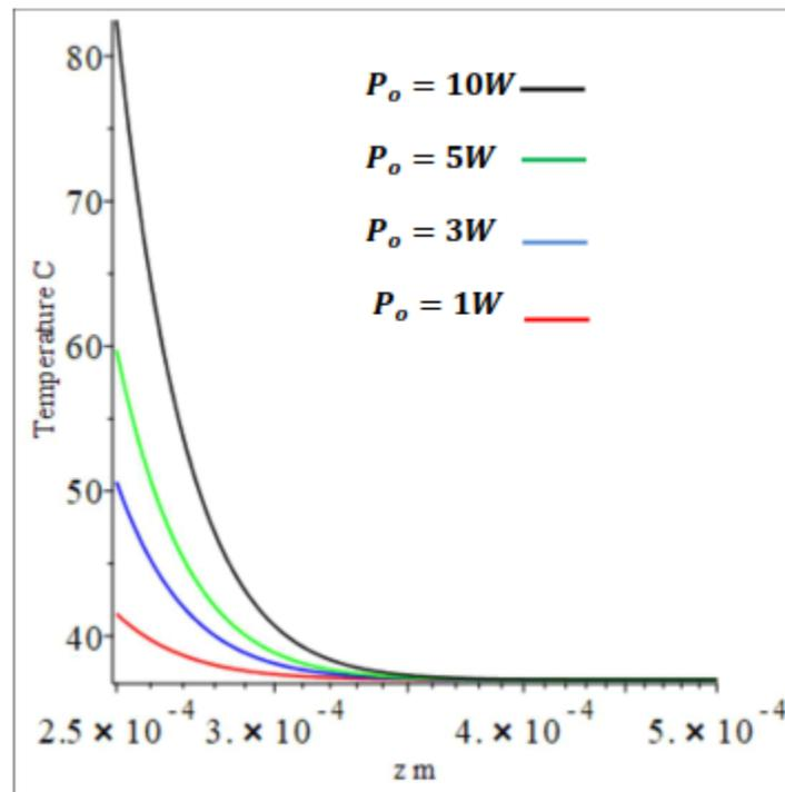
**Figure 3.** Radial temperature distribution with depth into the tumor tissue  $z$  for different laser power  $P_o$  at the center of the laser beam band ( $r = 0$ ) and irradiation time  $t = 0.5$  sec .
