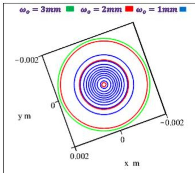
**Figure 7.** Filled temperature contours, represent the relation between spot size of laser beam and temperature, for the case of laser beam focus on the surface of tumor tissue.
