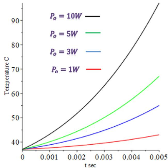
**Figure 4.** Radial temperature distribution against irradiation time  $t$  for beam focusing at the surface of tumor tissue  $z = 0$  with different laser power  $P_0$  and at the center of the laser beam band ( $r = 0$ ).
