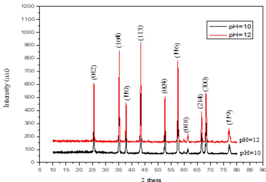
**Figure 4.** XRD patterns of  $\alpha$ - $\text{Al}_2\text{O}_3$  particles prepared at different pH values at  $1300^\circ\text{C}$ .
