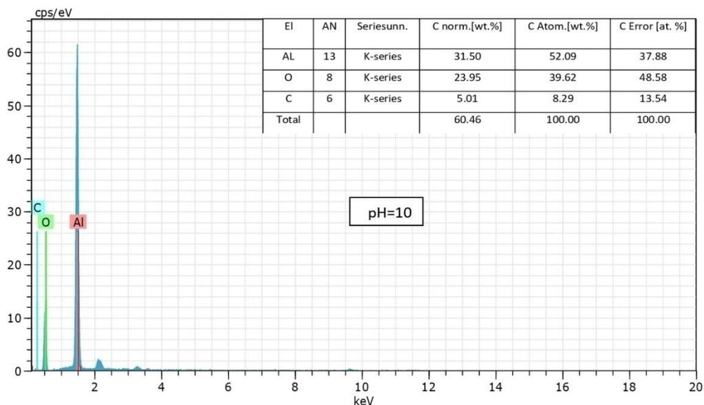
Figure 7.EDS spectrum of  $\alpha$ -Al<sub>2</sub>O<sub>3</sub> powder prepared at pH=10.
