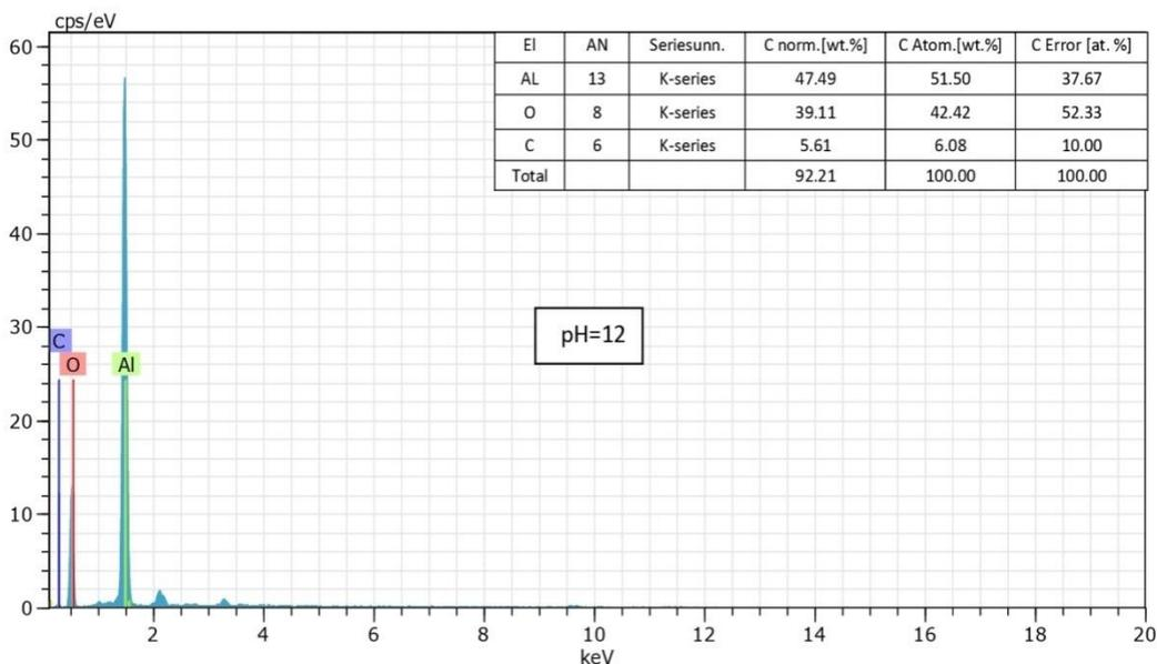
Figure 8.EDS spectrum of  $\alpha$ -Al<sub>2</sub>O<sub>3</sub> powder prepared at pH=12.
