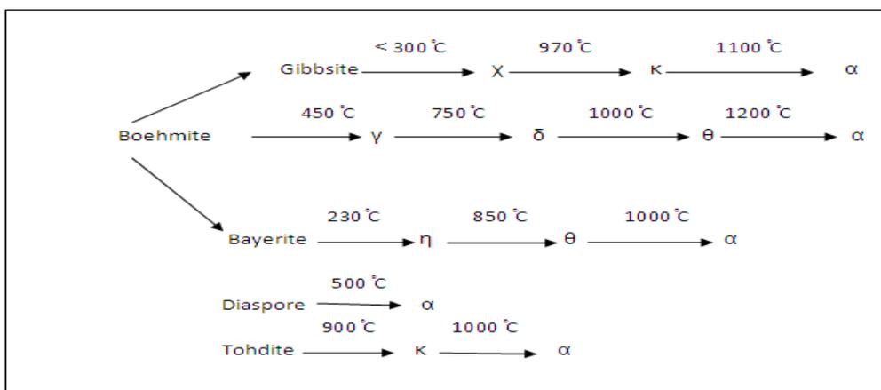
**Figure 2.** Phase transformation of transition alumina.
