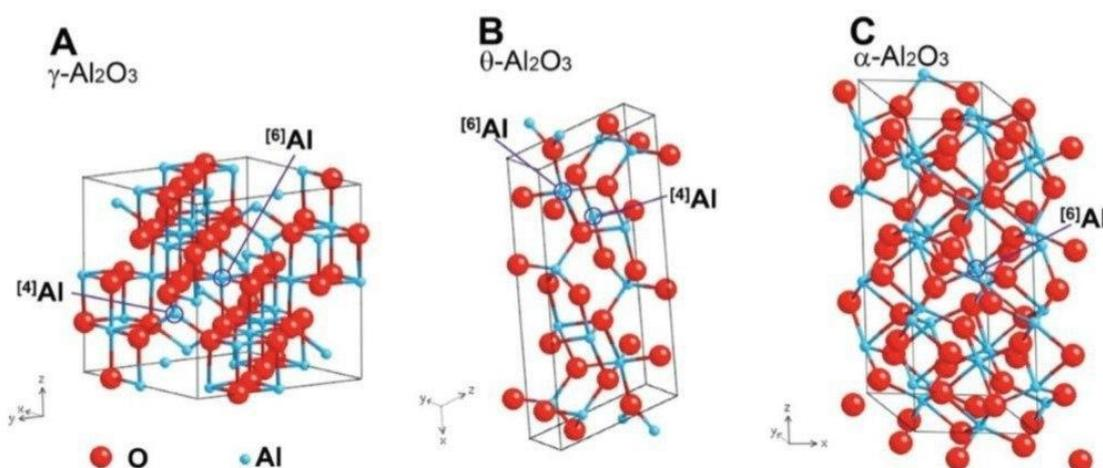
**Figure 1.** Molecular structures of alumina phases; A:  $\gamma$ - $\text{Al}_2\text{O}_3$ ; B:  $\theta$ - $\text{Al}_2\text{O}_3$ ; C:  $\alpha$ - $\text{Al}_2\text{O}_3$ .
