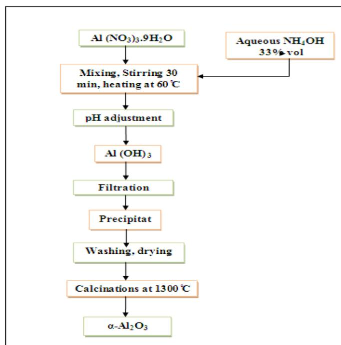
Figure 3. Flowchart of synthesis  $\alpha$ -Al<sub>2</sub>O<sub>3</sub> by co-precipitation process.
