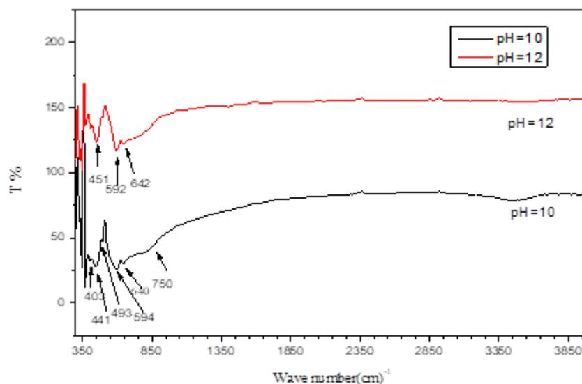
**Figure 5.** FT-IR spectroscopy of  $\alpha$ - $\text{Al}_2\text{O}_3$  particles prepared at different pH values (10, 12) at  $1300^\circ\text{C}$ .
