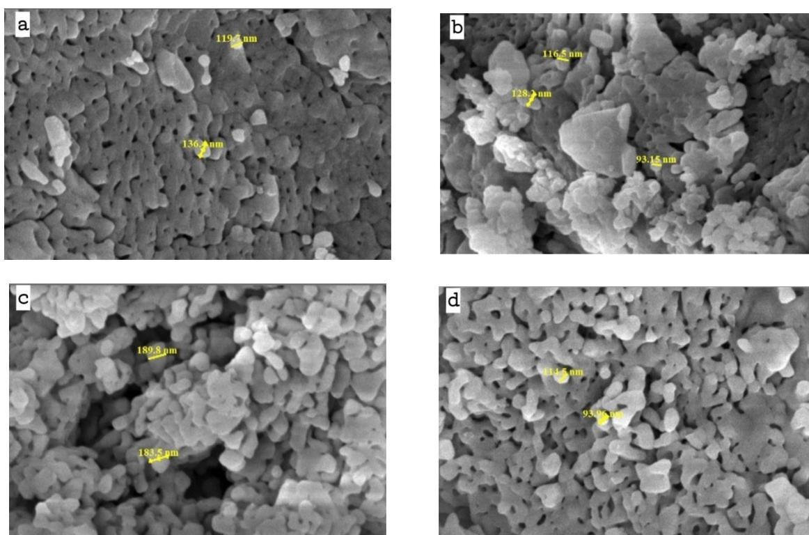
**Figure 6.** SEM images of  $\alpha$ - $\text{Al}_2\text{O}_3$  powders prepared at  $1300^\circ\text{C}$  (a, b, at pH=10): (c, d, at pH=12).
