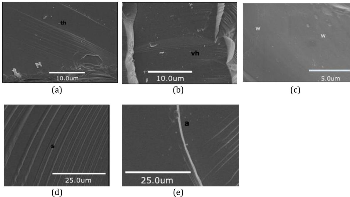
**Figure 1.** Example of microscale fractography features where (a) twist hackles (*th*), (b) velocity hackles (*vh*), (c) Wallner line (*w*), (d) striation (*s*), and (e) arrest line (*a*).
