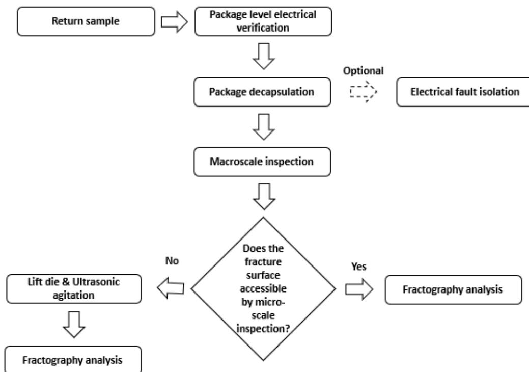
**Figure 2.** Fractography failure analysis flow.
