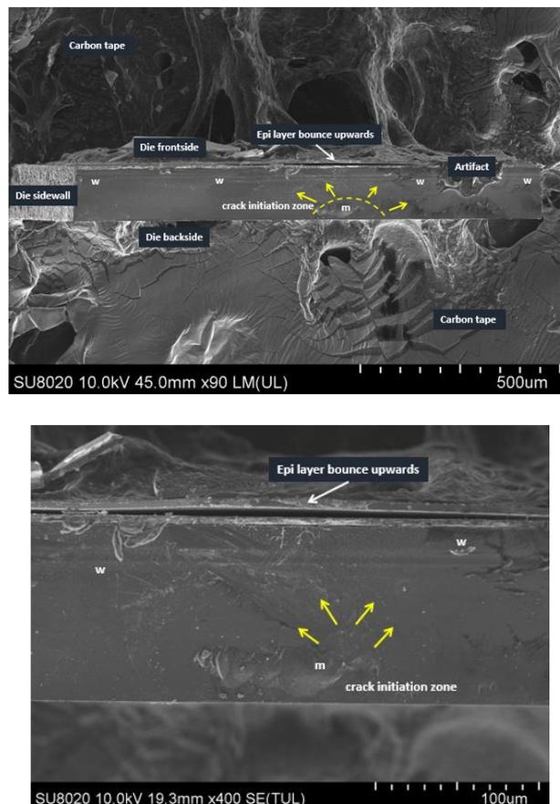
**Figure 7.** [Left] Micrograph shows the fracture chip vertically stick using carbon tape onto the scanning electron microscope (SEM) stud thereby the fracture surface is better to expose for viewing. [Right] Micrograph is a close up on fracture feature of a mirror (m) and Wallner (w) lines; LED epitaxial layer observed bouncing upwards.
