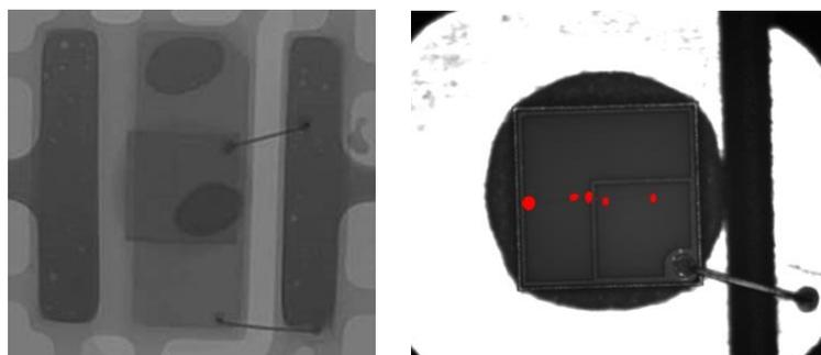
**Figure 6.** [Left] The x-ray radiograph top view shown insufficient epoxy adhesive underneath the chip. [Right] Photon emission microscope (PEM) is an electrical fault isolation technique used to review hot spots.
