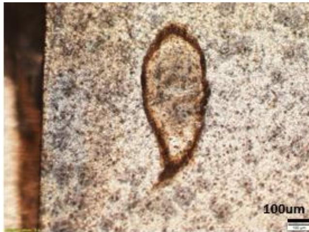
**Figure 3.** An optical representation of chemical damage on metallization if chemical residual not wholly removed.
