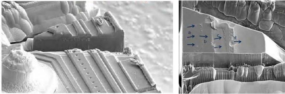
**Figure 5.** A cheesecake-like isolated island creates by the focus-ion beam (FIB). It reprinted with permission from [9] and not according to the scale for protecting proprietary information.
