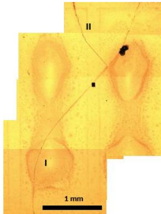
**Figure 4.** Macroscopic inspection of the sample reveals primary crack (line I) occurs before secondary crack (line II). The focus area to look for crack initiation zone will be on the surface of line I.
