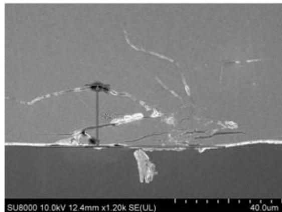
**Figure 8.** An example of the crack initiation from chip backside cross-sectional view.
