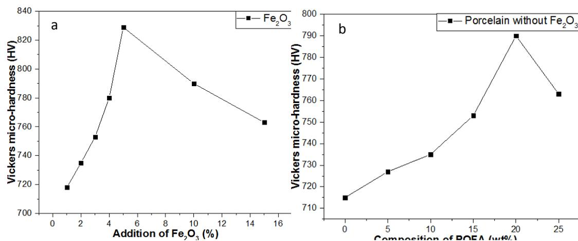
**Figure 5.** Vickers microhardness of Porcelain made with and without the addition of  $\text{Fe}_2\text{O}_3$ .
