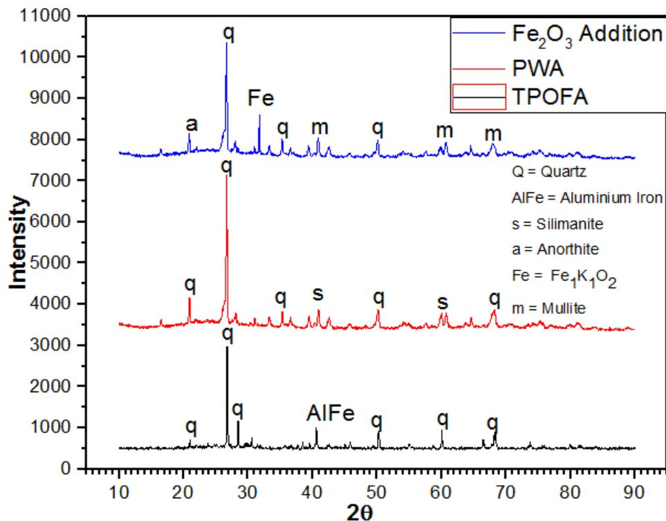
**Figure 2.** XRD pattern of treated POFA (TPOFA), porcelain without the addition of  $\text{Fe}_2\text{O}_3$  (PWA) and porcelain with the addition of  $\text{Fe}_2\text{O}_3$ .
