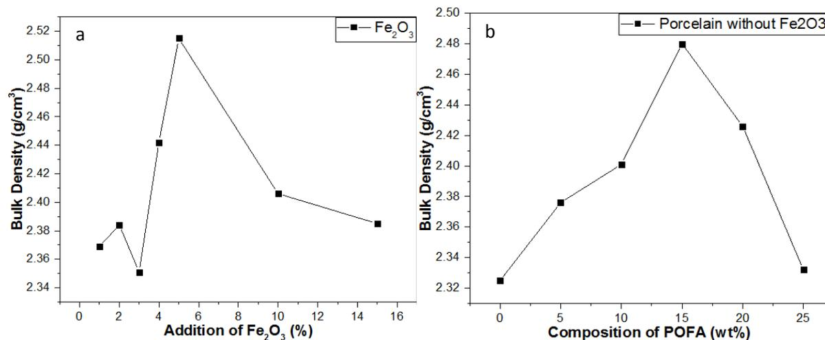
**Figure 4.** The bulk density of porcelain with and without the addition of Fe<sub>2</sub>O<sub>3</sub>.
