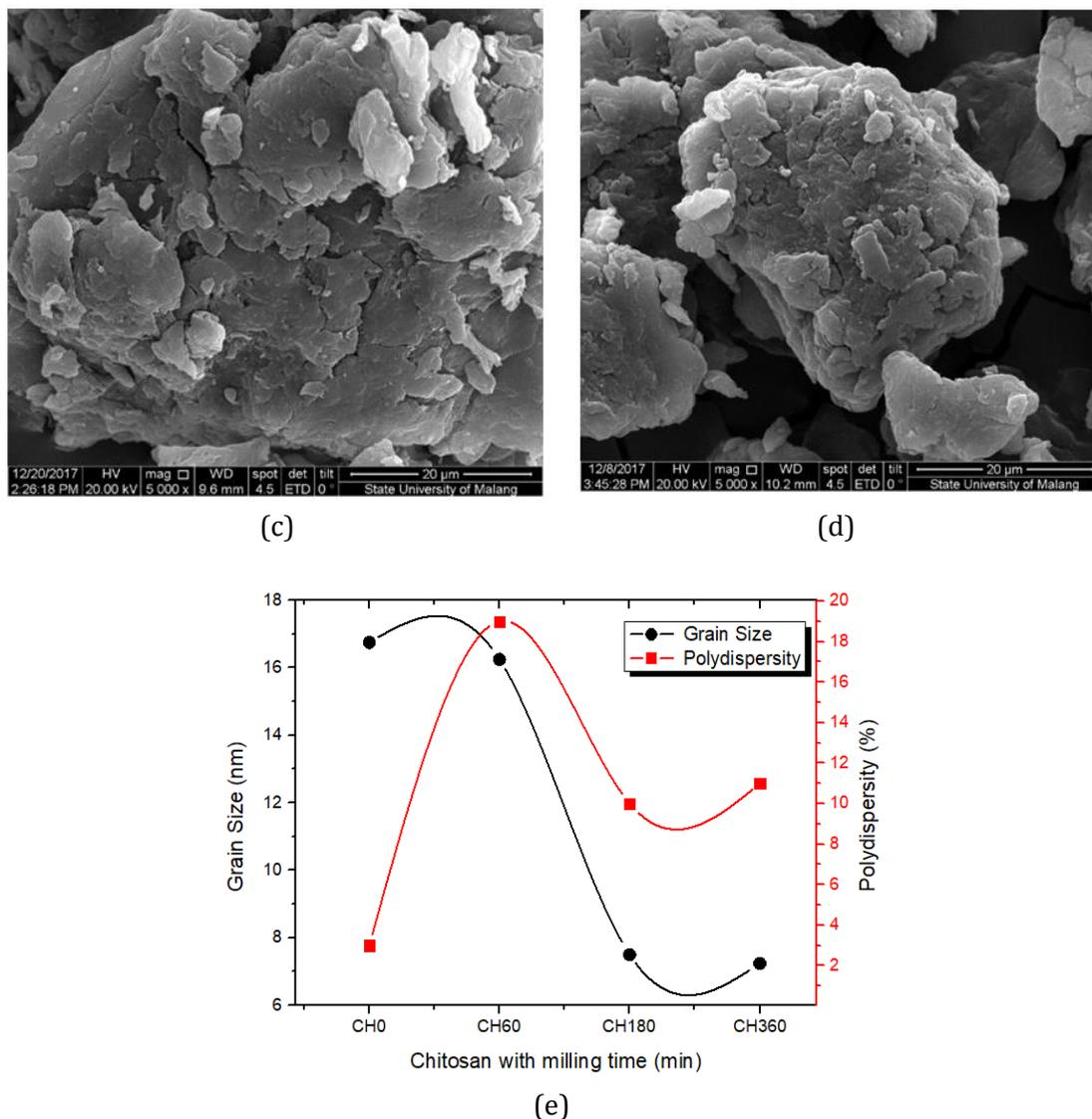
**Figure 1.** SEM images of (a) CH0, (b) CH60, (c) CH180, (d) CH360, (e) grain size and polydispersity.
