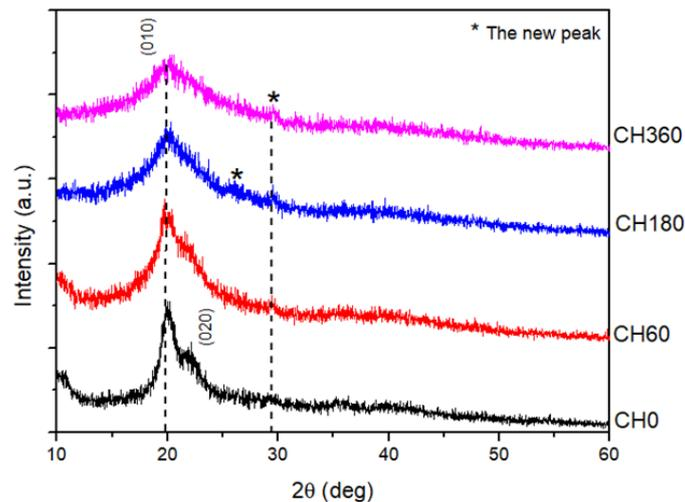
**Figure 3.** XRD patterns of CH0, CH60, CH180 and CH360.
