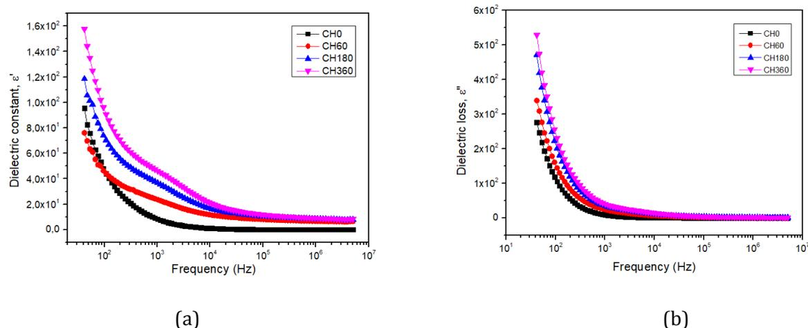
**Figure 5.** Frequency-dependent plot of permittivity for CH0, CH60, CH180 and CH360, (a) dielectric constant, (b) dielectric loss at RT.
