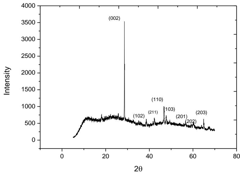
Figure 2. XRD patterns of  $\gamma$ -MnS thin film.
