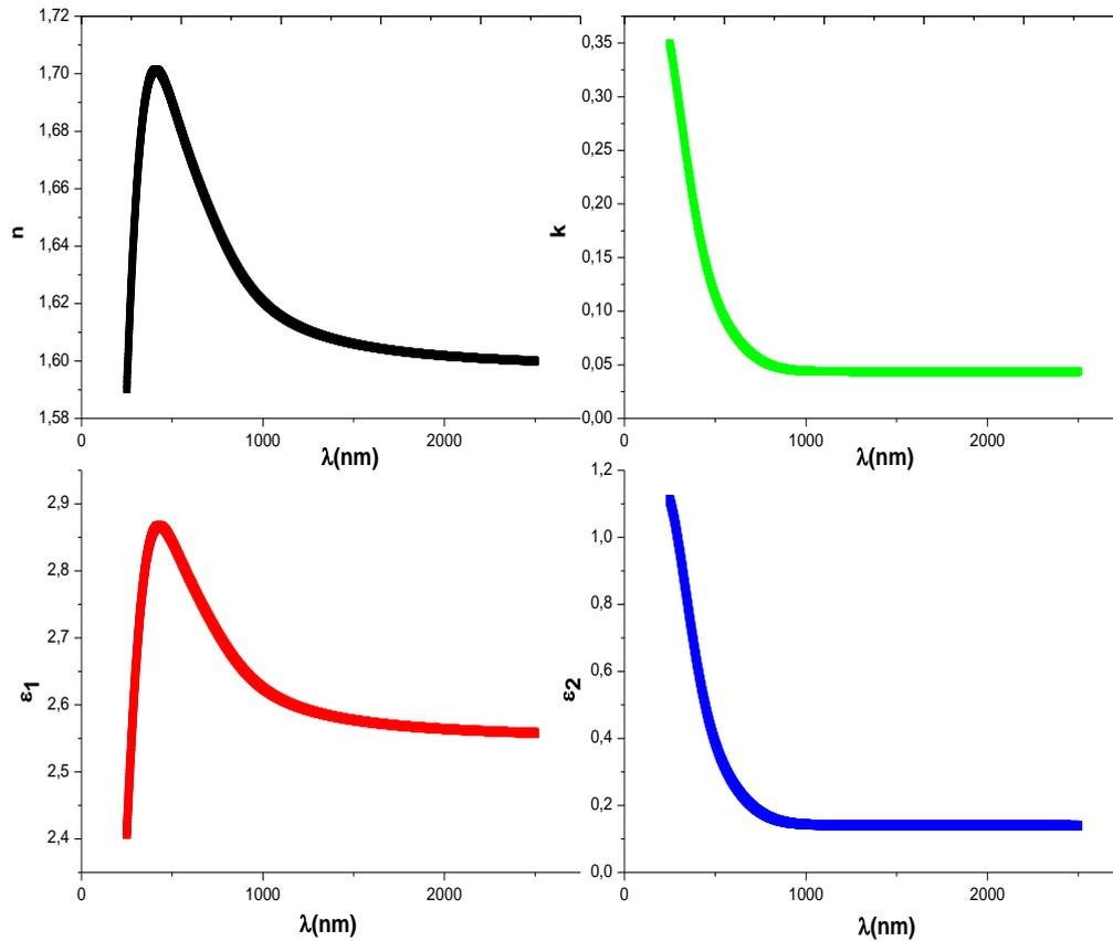
**Figure 7.** Optical constants ( $n$ ,  $k$ ,  $\epsilon_1$ ,  $\epsilon_2$ ) versus energy wavelength of  $\gamma$ -MnS thin films.
