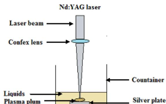
**Figure 1.** Schematic diagram of laser ablation in liquid.
