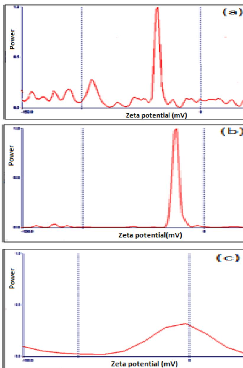
**Figure 4.**  $\zeta$ -potential of silver NPs prepared by laser ablation in acetone, toluene, and cyclohexane, respectively.
