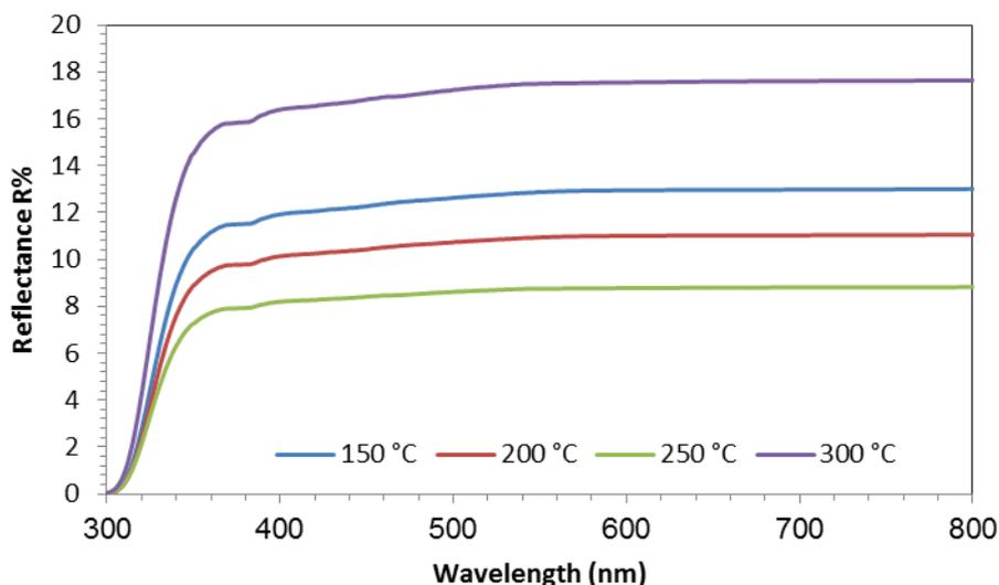
**Figure 5.** Reflectance as a function of wavelength range under two substrate temperatures.
