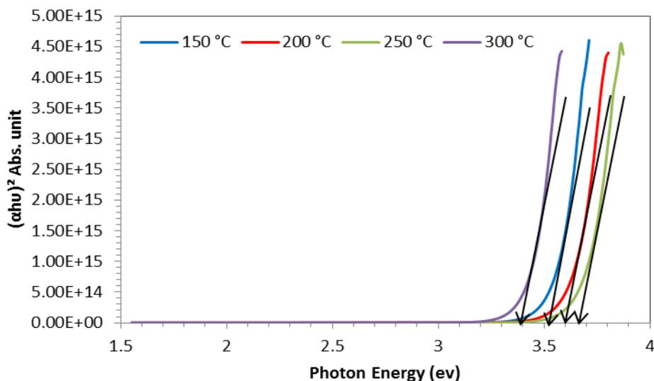
**Figure 4.** The optical band-gap energy as a function of photon energy for two substrate temperatures.
