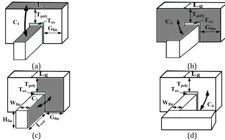
**Figure 3.** Gate Parasitic Capacitance (a) Parasitic Capacitance  $C_1$  at top of gate and top of the fin (b) Parasitic Capacitance  $C_2$  at gate sidewall and top of the fin (c) Parasitic Capacitance at  $C_3$  gate sidewall and fin sidewall (d) Parasitic Capacitance  $C_4$  at gate sidewall and S/D sidewall.
