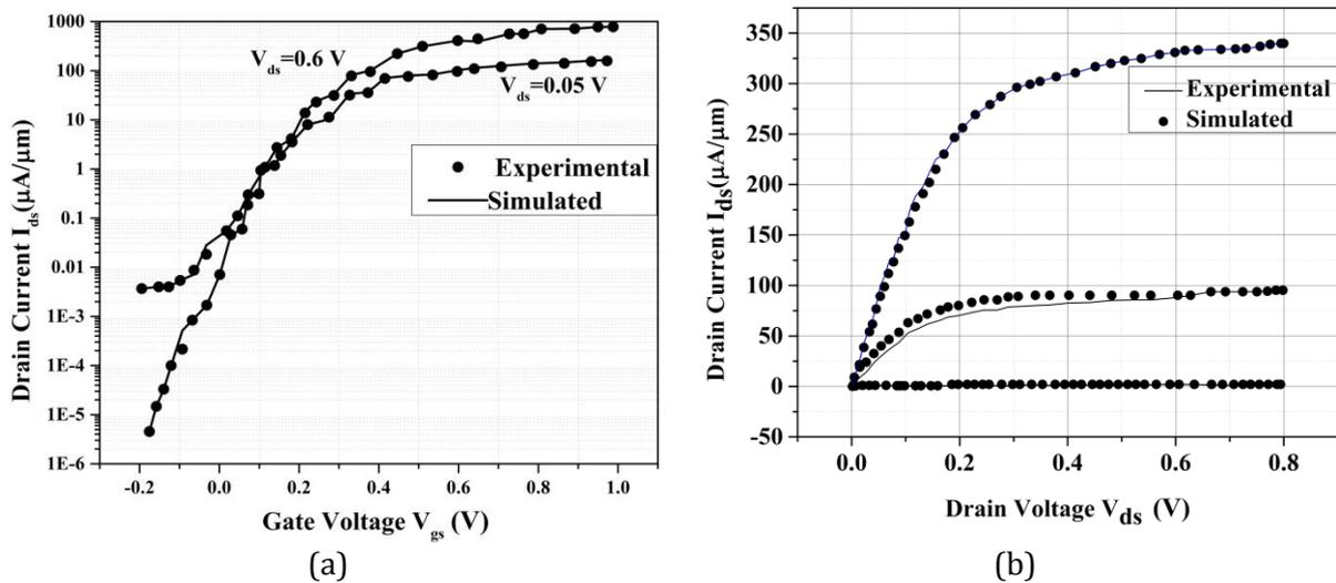
**Figure 2.** Calibration of  $\text{In}_{0.53}\text{Ga}_{0.47}\text{As}$  nFinFET with  $L_g = 50 \text{ nm}$  (a)  $I_{ds}$ - $V_{gs}$  transfer characteristics during different drain bias (b)  $I_{ds}$ - $V_{ds}$  output characteristics during different gate bias.
