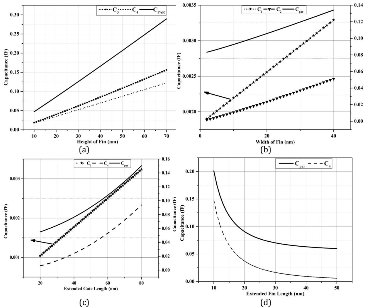
**Figure 6.** Gate Parasitic Capacitance (a) Parasitic Capacitance versus Height of fin (b) Parasitic Capacitance versus Width of fin (c) Parasitic Capacitance versus Extended Gate Length (d) Parasitic Capacitance versus Extended fin Length.
