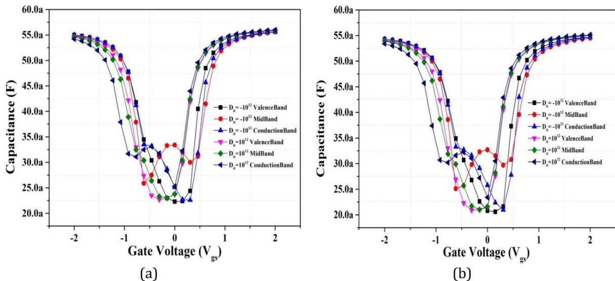
Figure 7. Gate Capacitance for InGaAs FinFET with  $D_{it} = 10^{12} \text{cm}^{-2} \text{eV}^{-1}$  (a)  $L_{un} = 6 \text{ nm}$  (b)  $L_{un} = 9 \text{ nm}$ .
