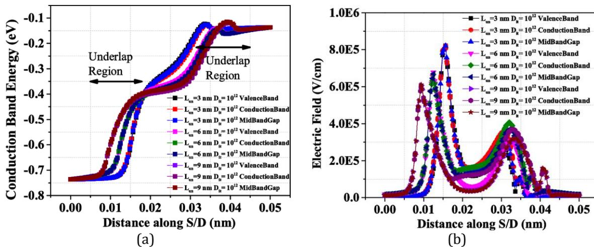
Figure 5. Conduction Band Energy and Electric Field for  $D_{it}= 10^{12}\text{cm}^{-2}\text{eV}^{-1}$  at different energy trap levels.
