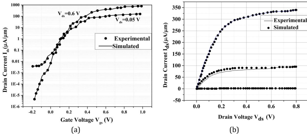
**Figure 2.** Calibration of  $\text{In}_{0.53}\text{Ga}_{0.47}\text{As}$  nFinFET with  $L_g = 50 \text{ nm}$  (a)  $I_{ds}$ - $V_{gs}$  transfer characteristics during different drain bias (b)  $I_{ds}$ - $V_{ds}$  output characteristics during different gate bias.
