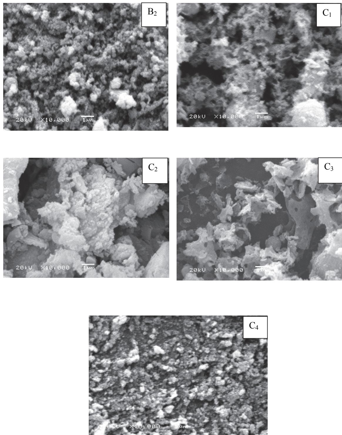
**Figure 3.** SEM Analysis of synthesized pure nano zinc oxide by both chemical and green synthesis methods: (A) chemical, (B<sub>1</sub>) olive fresh, (B<sub>2</sub>) guava fresh, (C<sub>1</sub>) olive dry, (C<sub>2</sub>) guava dry, (C<sub>3</sub>) fig dry and (C<sub>4</sub>) lemon dry.
