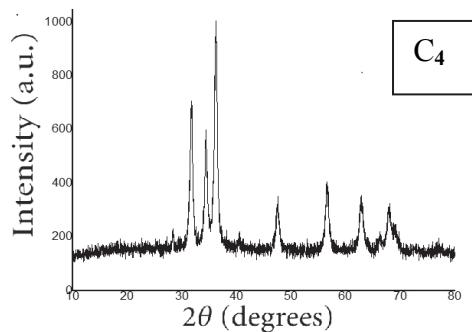
**Figure 2.** XRD spectrums of synthesized pure nano zinc oxide using both chemical and green synthesis methods: (A) chemical, (B<sub>1</sub>) olive fresh, (B<sub>2</sub>) guava fresh, (C<sub>1</sub>) olive dry, (C<sub>2</sub>) guava dry, (C<sub>3</sub>) fig dry and (C<sub>4</sub>) lemon dry.
