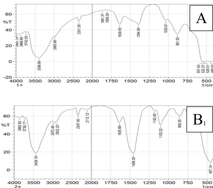
**Figure 5.** FTIR spectroscopy of chemical (A) and green (B<sub>1</sub>) synthesis methods.
