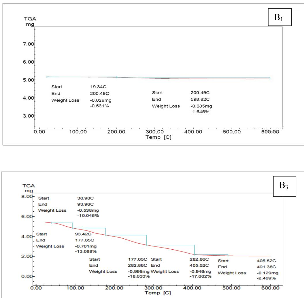
**Figure 6.** Thermo gravimetric analysis (TGA) for ZnO nanoparticles: (A) chemical, (B<sub>1</sub>) green synthesis methods calcinated ZnO nanoparticles at 500°C for 2 hr and (B<sub>3</sub>) green synthesis methods without calcination of ZnO paste.
