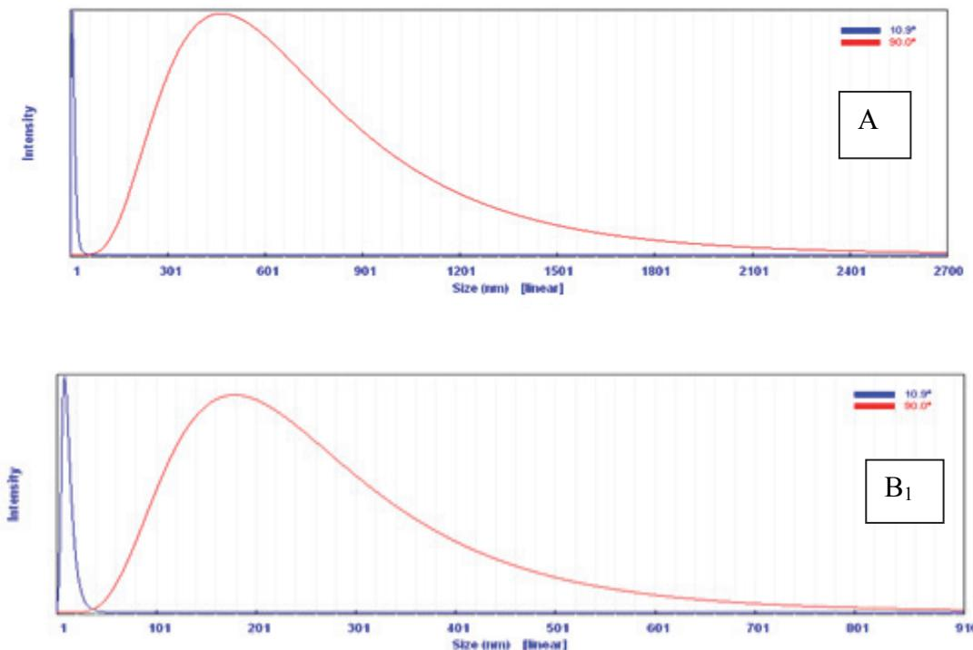
**Figure 7.** Particle Size Analysis (PSA) for ZnO nanoparticles (A) chemical and (B<sub>1</sub>) green synthesis methods.
