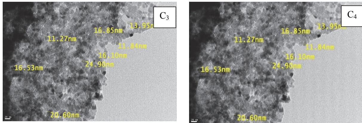
**Figure 4.** TEM images of the ZnO nanoparticles synthesized using both chemical and green synthesis methods: (A) chemical, (B<sub>1,1</sub>, B<sub>1,2</sub>) olive fresh, (B<sub>2</sub>) guava fresh, (C<sub>1</sub>) olive dry, (C<sub>2</sub>) guava dry, (C<sub>3</sub>) fig dry and (C<sub>4</sub>) lemon dry.
