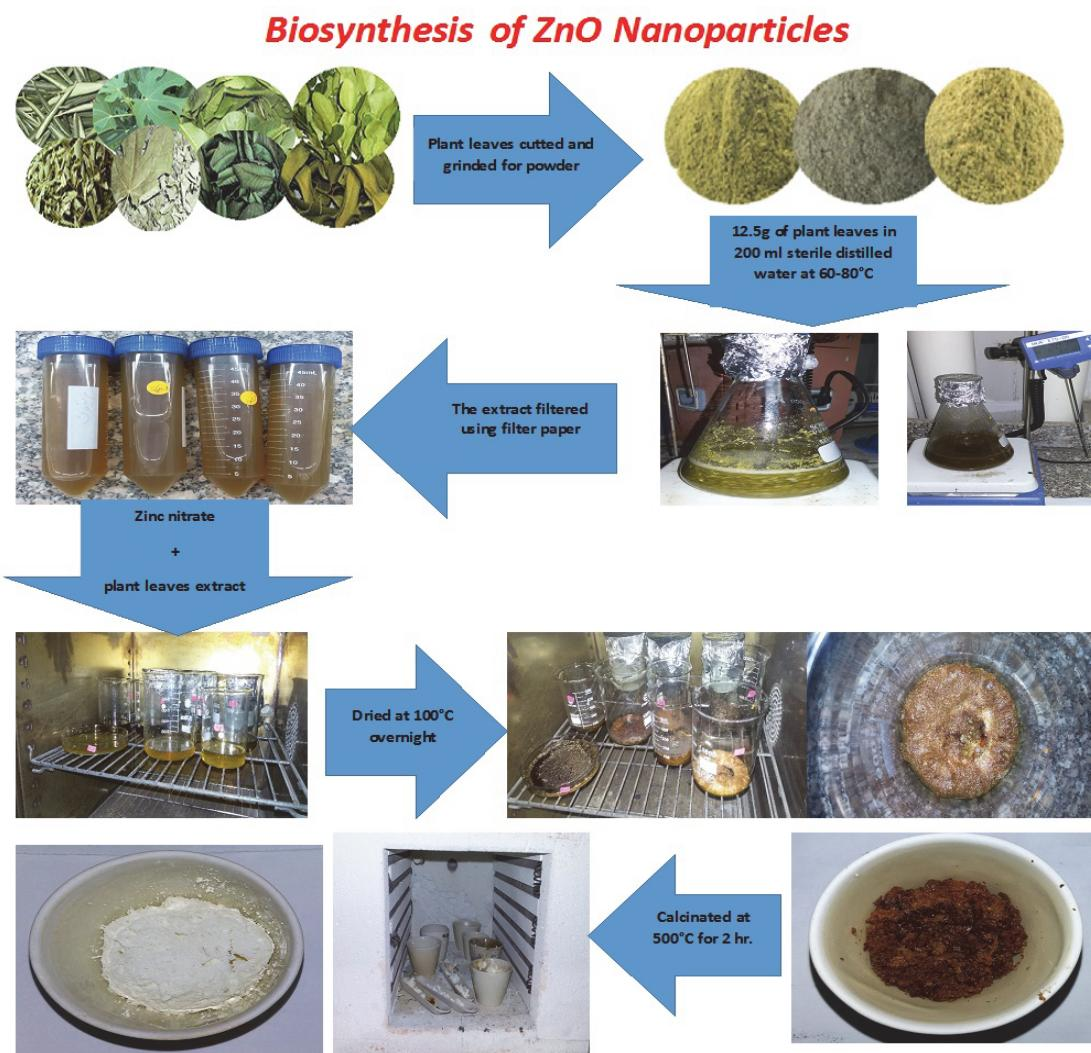
**Figure 1.** Biosynthesis of ZnO nanoparticles schematic diagram.
