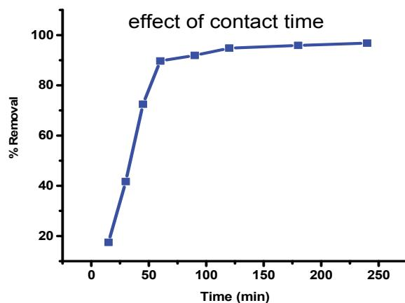
**Figure 8.** Effect of contact time on phenol removal onto green synthesized ZnO-NPs.
