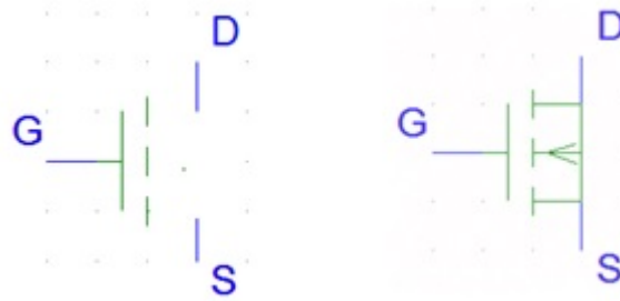
Fig. 1: (a): Switch showing the Stuck-open fault i.e the transistor will be disconnected from the circuit and (b): Switch showing the Stuck-short fault i.e short between Source (S) and Drain (D) terminals
