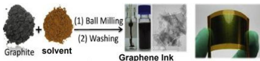
**Figure 17.** The processes that have been used to prepare graphene ink [161].
