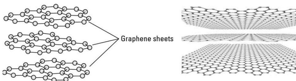
**Figure 8.** Graphene sheets that exfoliated from graphite [32].
