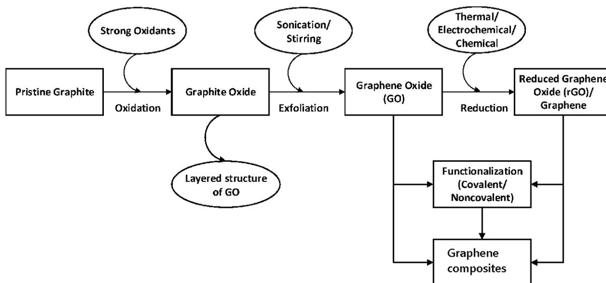
Figure 14. Schematic representation of the graphene functionalization [72-75].
