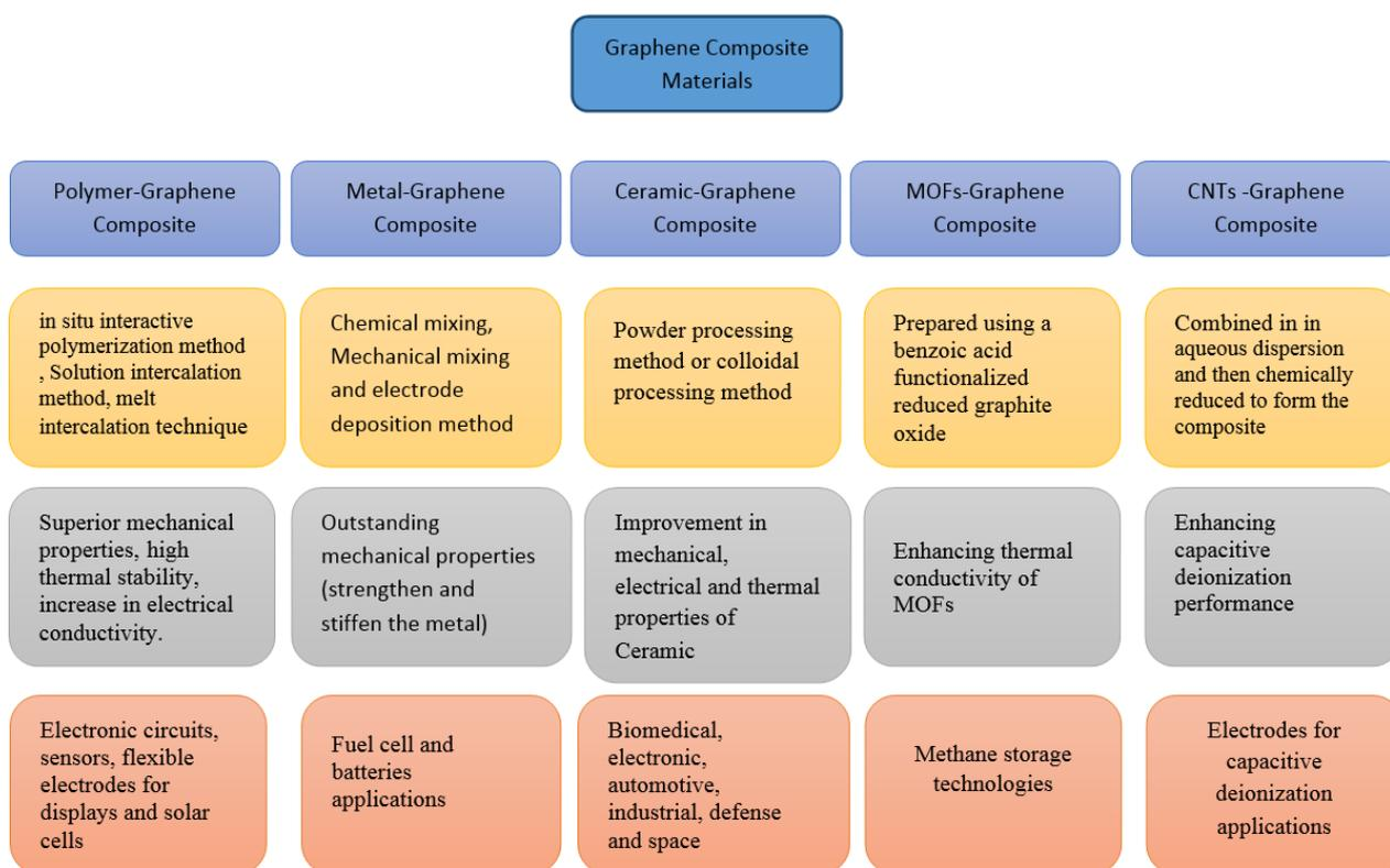
**Figure 12.** Types, fabrication, properties and applications of Graphene Composite Materials [60-65].
