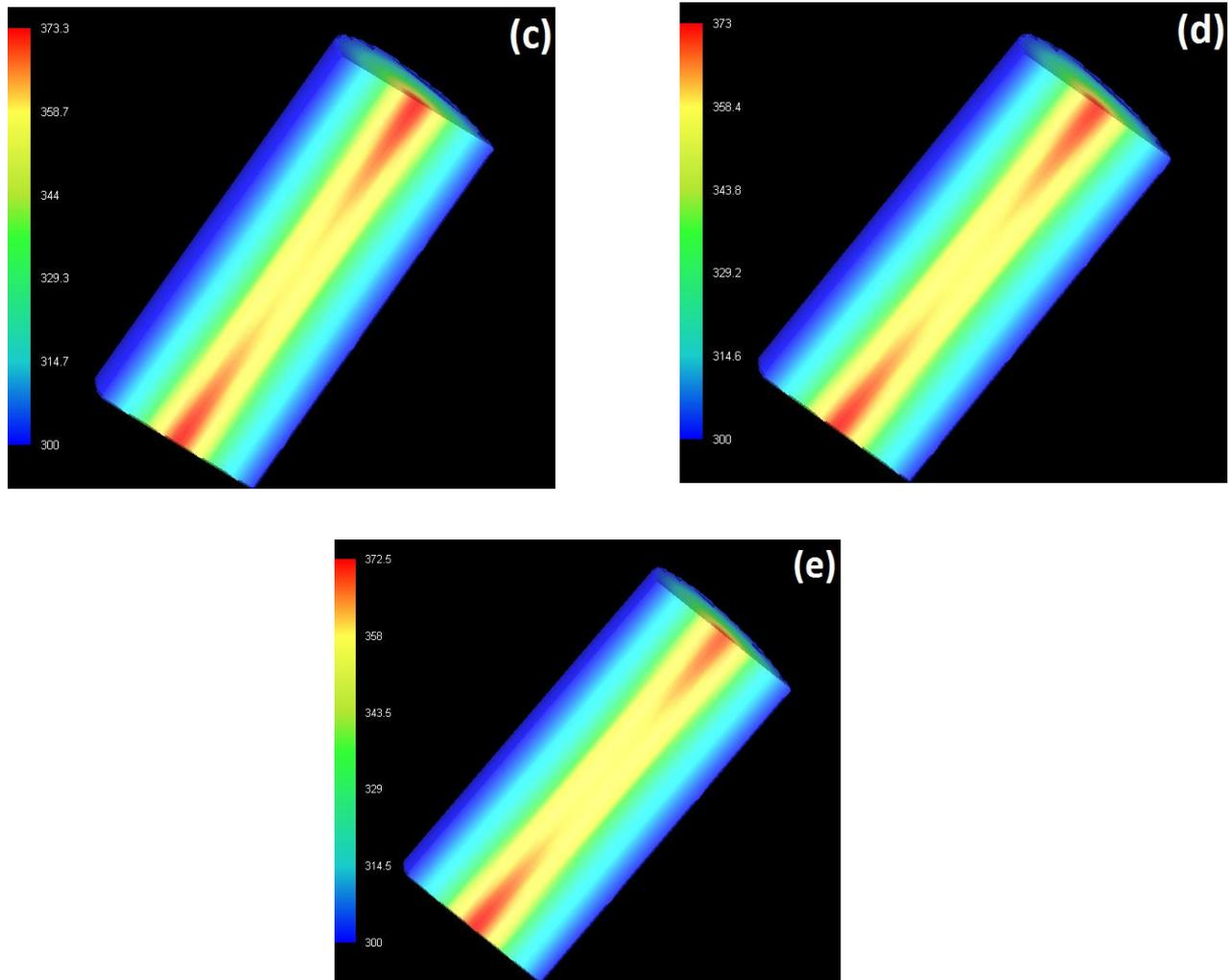
**Figure 2.**  $\frac{1}{2}$  Rod simulation thermal model for (a) Gaussian, (b)  $N = 4$ , (c)  $N = 6$ , (d)  $N = 10$ , and (e)  $N = 30$ .
