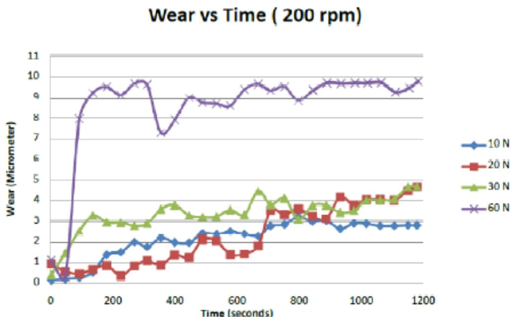
**Figure 5.** Wear vs Time for 200 rpm [43].
