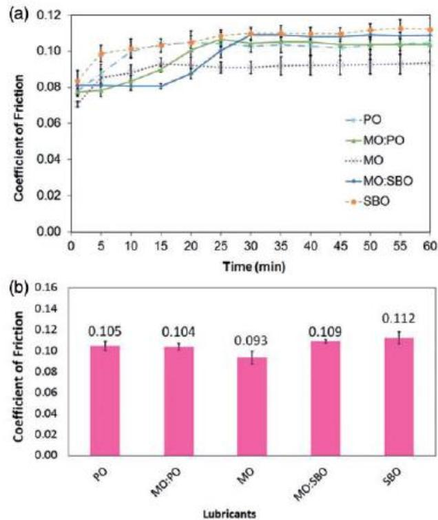
**Figure 10.** (a) Average coefficient of friction versus time for palm oil (PO), soybean oil (SBO), mineral oil (MO) and their oil blends, and (b) coefficient of friction value at 60 min [47].
