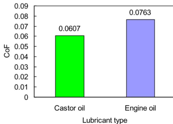
**Figure 11.** Coefficient of frictions of the investigated oils for wear test [48].
