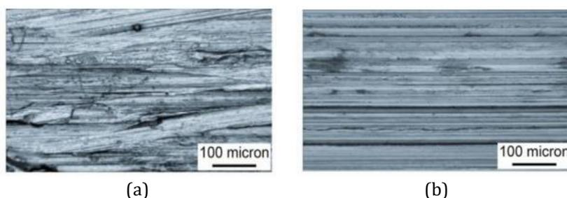
**Figure 6.** the wear groove at different speed of disk (a) at 0.4 m/s, (b) at 4.0 m/s [45].
