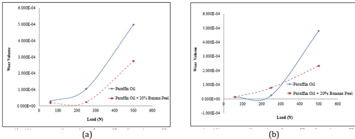
**Figure 8.** (a) wear scar diameter of paraffin oil and paraffin oil with 20% of banana peel at 500 rpm and (b) wear scar diameter of paraffin oil and paraffin oil with 20% of banana peel at 1000 rpm.
