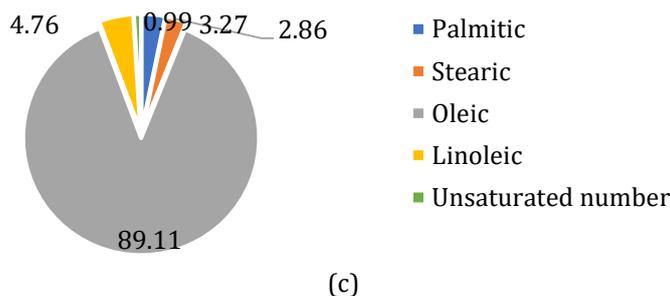
**Figure 1.** The fatty acid composition on three types of vegetable oils bio-based lubricant (a) Soybean, (b) Safflower, and (c) Sunflower [36].
