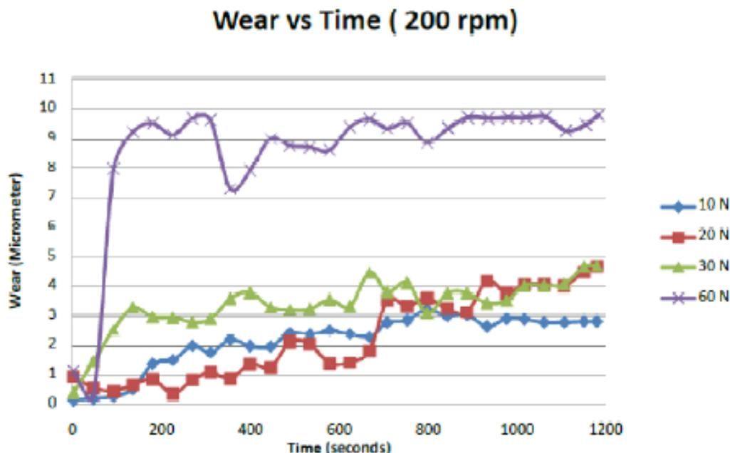
**Figure 5.** Wear vs Time for 200 rpm [43].
