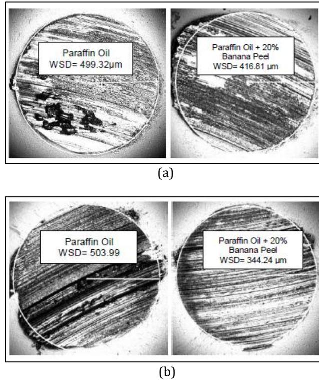
**Figure 7.** (a) Wear scar of paraffin oil and paraffin oil with 20% of banana peels with loads of 500 N at 500 rpm and (b) wear scar diameter of paraffin oil and paraffin oil with 20% of banana peel at 1000 rpm
