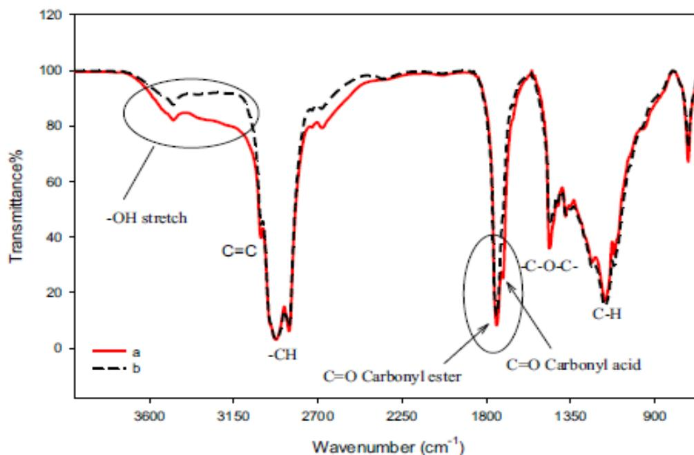
**Figure 2.** FTIR spectrums of (a) HFFA-CPO and (b) LFFA-CPO [39].
