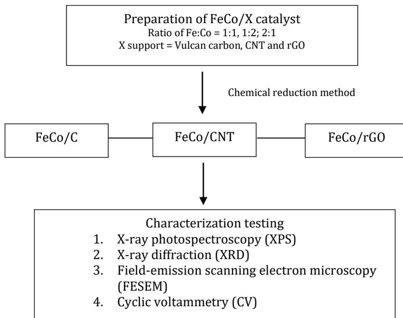
**Figure 1.** Schematic diagram of methodology.
