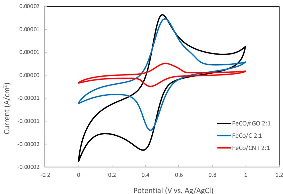
**Figure 5.** Cyclic voltammogram of FeCo/C, FeCo/CNT and FeCo/rGO samples in an O<sub>2</sub>-saturated 0.5 M H<sub>2</sub>SO<sub>4</sub> solution.
