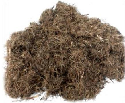
**Figure 1.** Oil palm Mesocarp fibre 10-15 mm in length.
