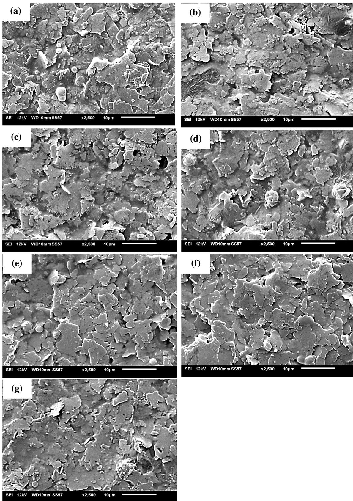
**Figure 5.** SEM micrograph of printed silver cured at different temperature: (a) room temperature, (b) 60°C, (c) 80°C, (d) 100°C, (e) 120°C, (f) 130°C, and (g) 140°C.
