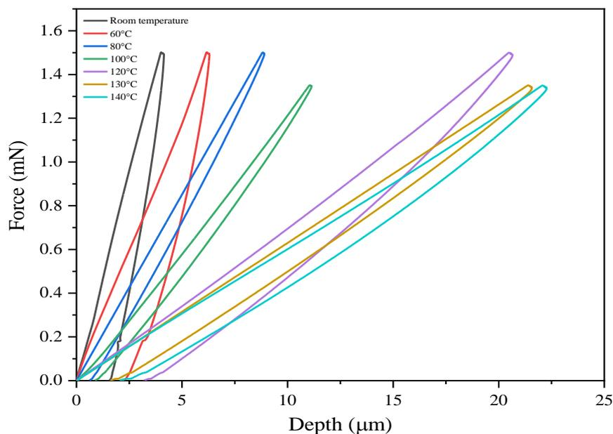
**Figure 7.** Nanoindentation load-displacement of silver at the different curing temperature.
