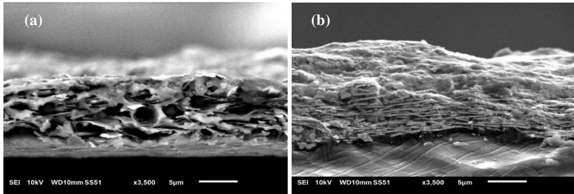
**Figure 6.** SEM micrograph of a cross-sectional view of printed silver cured at different temperatures: (a) room temperature and (b) 120°C.
