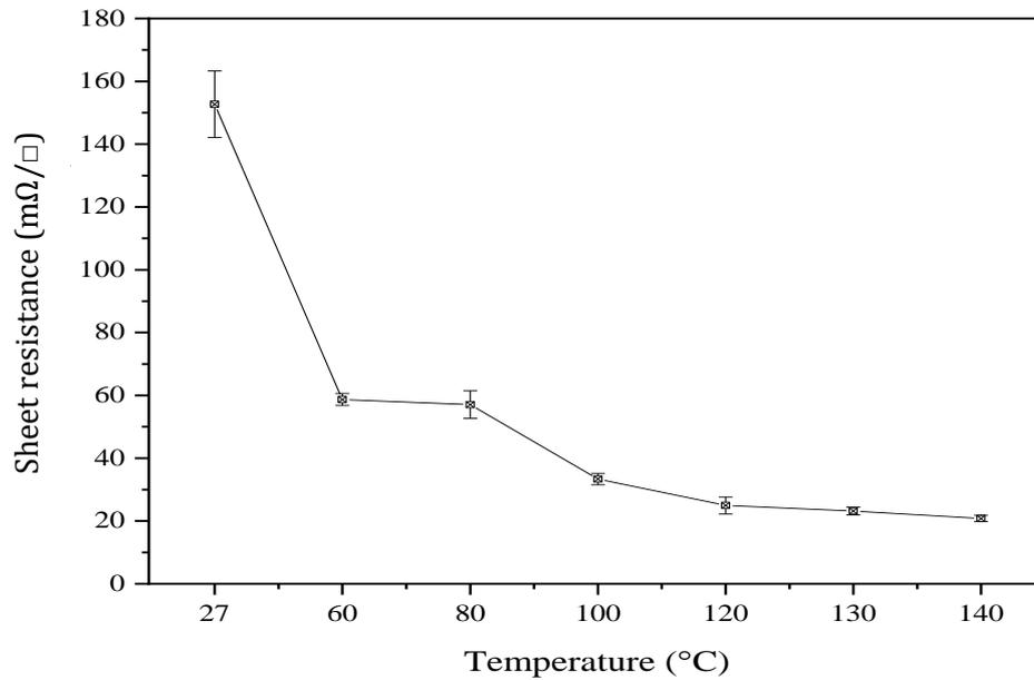
**Figure 3.** Effect of temperature on the conductivity of silver.
