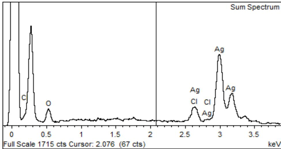
Figure 2. EDX spectrum of silver conductive ink.
