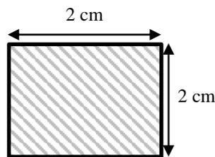
**Figure 1.** The test pattern of printed silver on TPU substrate.
