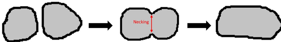
**Figure 4.** The grain diffusion initiates when temperature elevated
