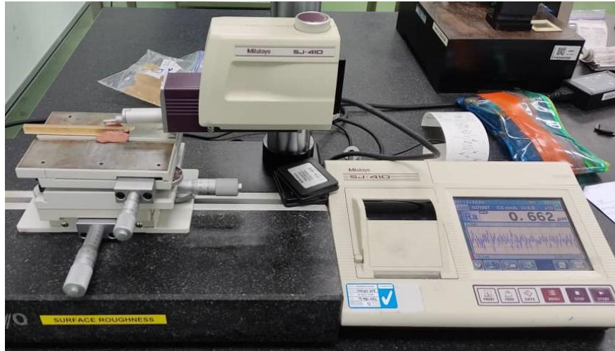
Figure 5. Setup experiment for surface roughness.
