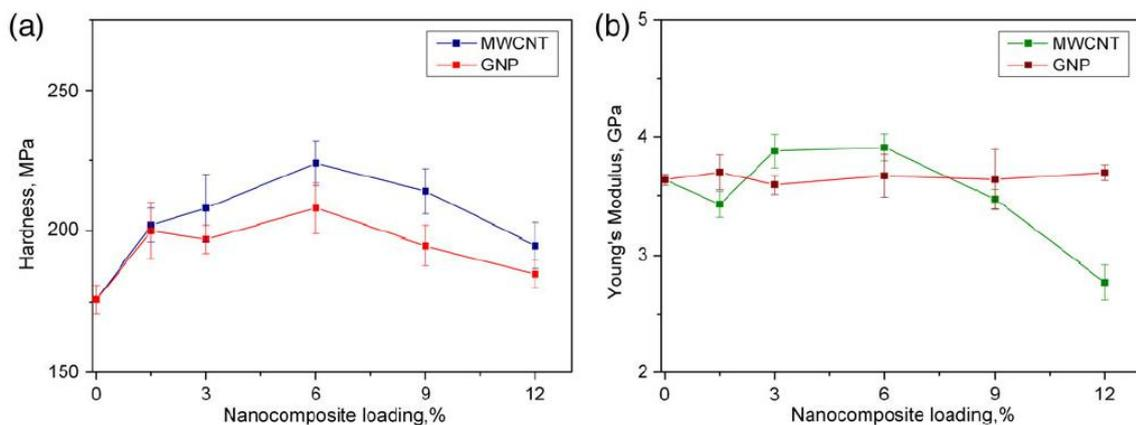
**Figure 7:** Mean values of (a) hardness and (b) Young's modulus of elasticity versus mono-filler content [11].
