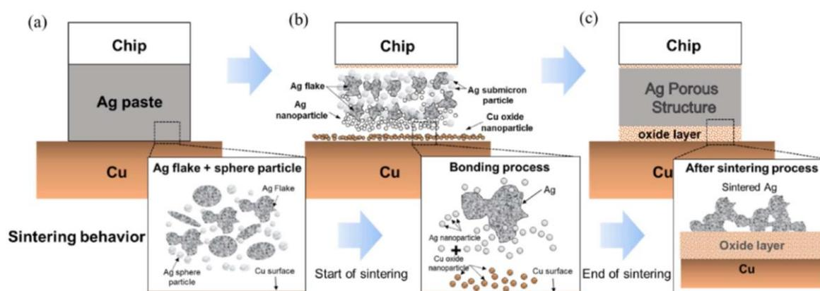
**Figure 2.** Bonding mechanism illustration of sintering Ag paste on Cu substrate, (a) before sintering; (b) start of sintering; (c) end of sintering [43].
