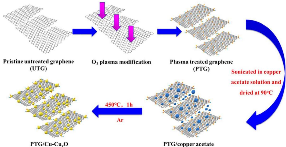
**Figure 1.** Schematic diagram of hybridization Cu-Cu<sub>x</sub>O nanoparticles on plasma-treated graphene (PTG) [47].
