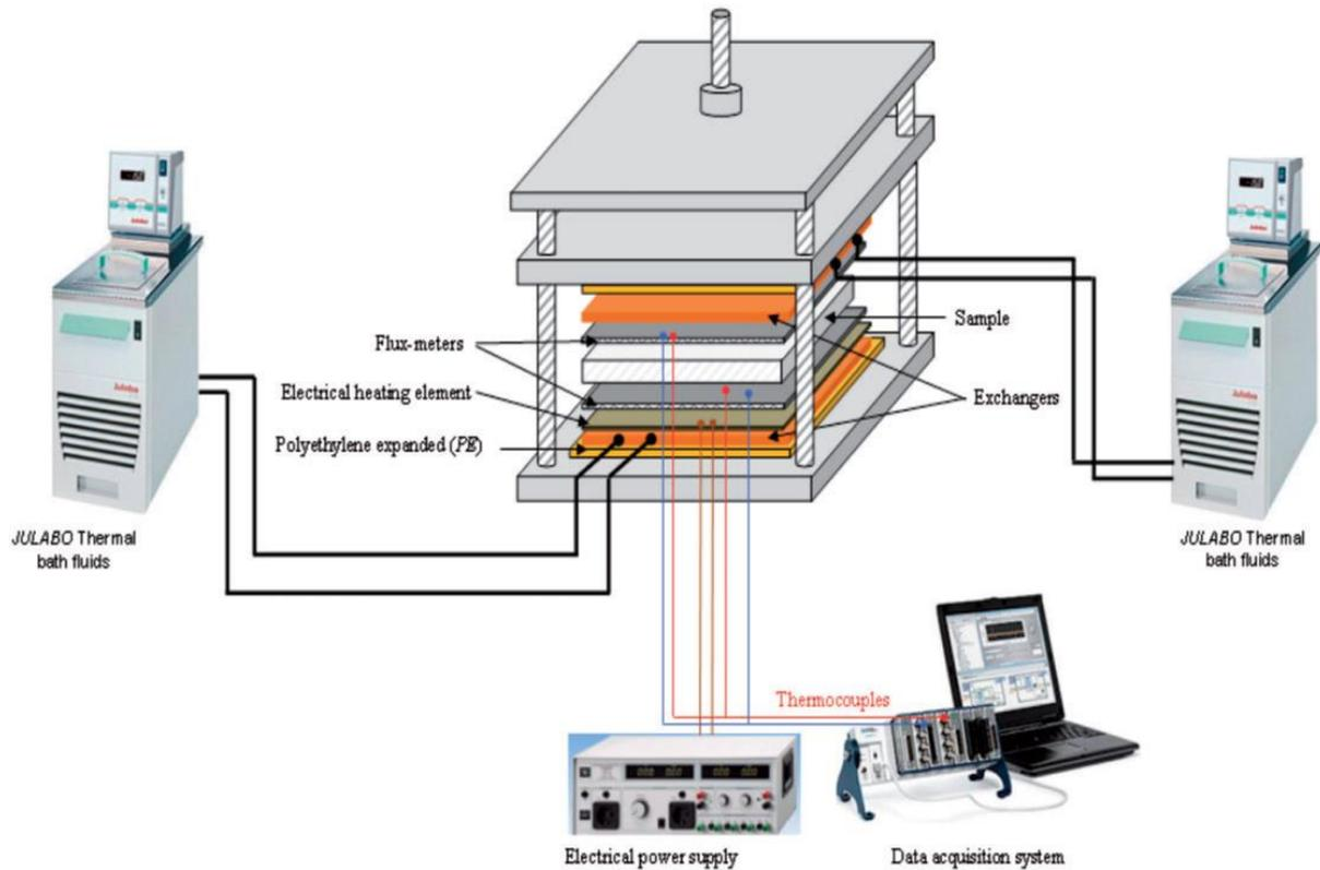
**Figure 4.** Experimental set-up of transient guarded hot plate method [49].
