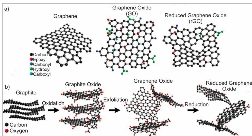
**Figure 5.** (a) Chemical structure illustration of graphene, graphene oxide, and reduced graphene oxide. (b) The synthesizing steps of reduced graphene oxide from the graphite material [58].
