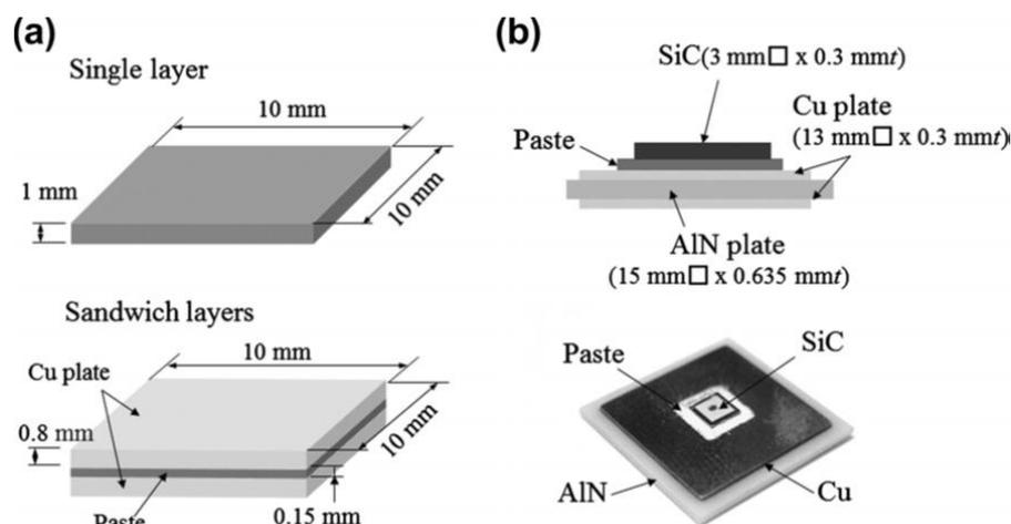
**Figure 3.** (a) Thermal conductivity measurement samples. Sandwiches of Cu-Cu substrate which the upper and lower were for intrinsic thermal conductivities and the lower is for those with thermal resistivity, respectively. (b) SiC die-attach setup and photograph [34].
