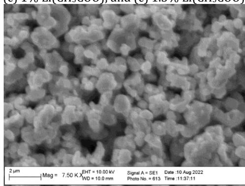
Figure 9. Morphology of BaTiO<sub>3</sub>/Si(100) thin film particles treated with 0.5% Lithium with a magnification of 7500 times the SEM image
