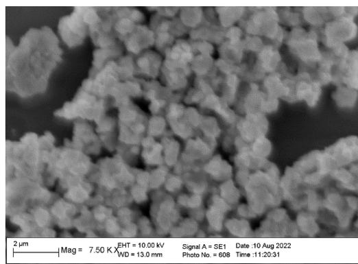
Figure 8. Morphology of the BaTiO<sub>3</sub>/Si(100) thin film particles not exposed to Lithium with a magnification of 7500 times the SEM image
