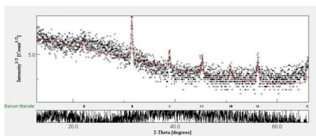
**Figure 1.** Diffraction pattern of  $\text{BaTiO}_3/\text{Si}(100)$  film without receptacle
