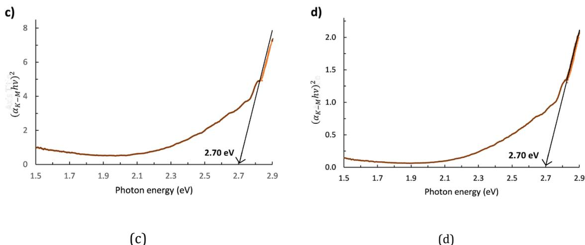
Fig. 7. Energy Gap: (a) 0% Li(CH<sub>3</sub>COO); (b) 0.5% Li(CH<sub>3</sub>COO); (c) 1% Li(CH<sub>3</sub>COO); and (c) 1.5% Li(CH<sub>3</sub>COO)
