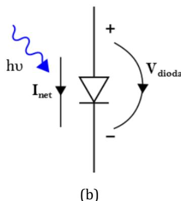
**Figure 16.** The arrangement of solar cells: (a) BaTiO<sub>3</sub>/Si(100) thin film-based solar cell structure in Lithium; (b) Electronic circuit of I-V curve characterization (without and with illumination)
