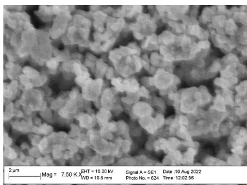
**Figure 11.** Morphology of BaTiO<sub>3</sub>/Si(100) thin film particles in 1.5% Lithium dispersed with a magnification of 7500 times the SEM image
