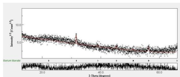
**Figure 2.**  $\text{BaTiO}_3/\text{Si}(100)$  film diffraction pattern with 0.5%  $\text{Li}(\text{CH}_3\text{COO})$
