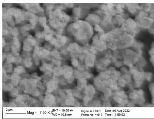
Figure 10. Morphology of BaTiO<sub>3</sub>/Si(100) thin film particles in 1% Lithium dispersed with a magnification of 7500 times the SEM image
