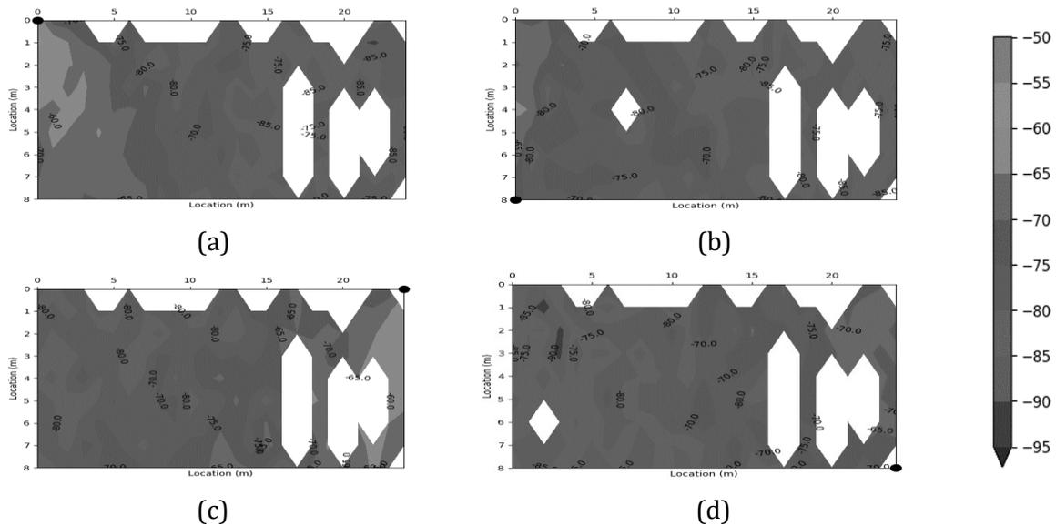
**Figure 4.** Average RSSI radio map representations for (a) receiver 1 (b) receiver 2 (c) receiver 3 (d) receiver 4
