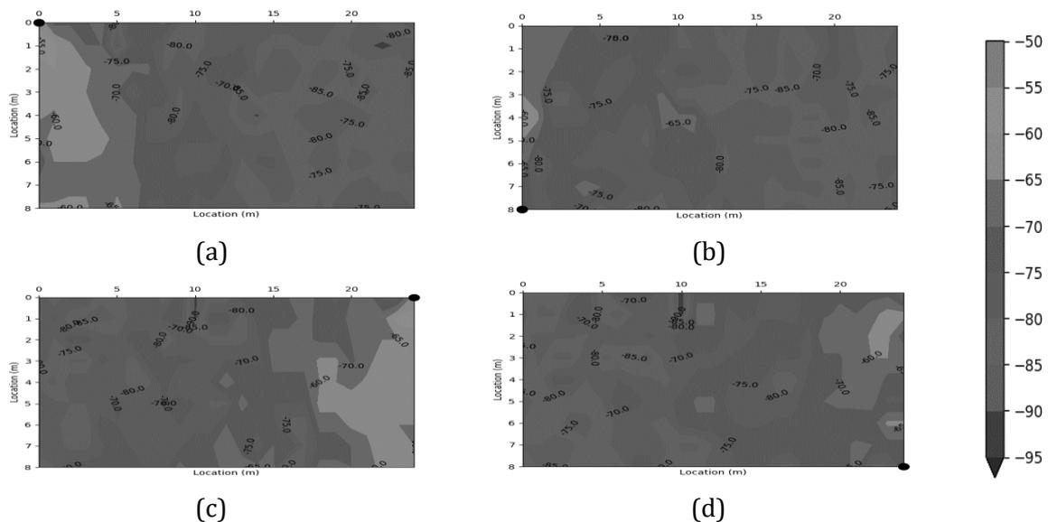
**Figure 5.** RBF interpolated (Gaussian) radio mappings based on 171 fingerprint locations for (a) receiver 1 (b) receiver 2 (c) receiver 3 (d) receiver 4
