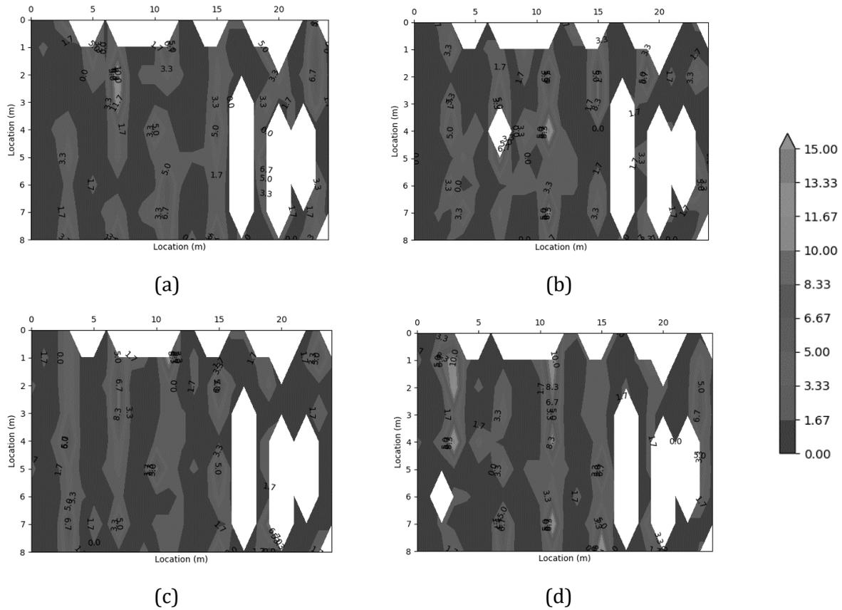
**Figure 6.** Errors plot for RBF interpolated (Inverse Multiquadric) radio mappings based on 171 fingerprint locations for (a) receiver 1 (b) receiver 2 (c) receiver 3 (d) receiver 4
