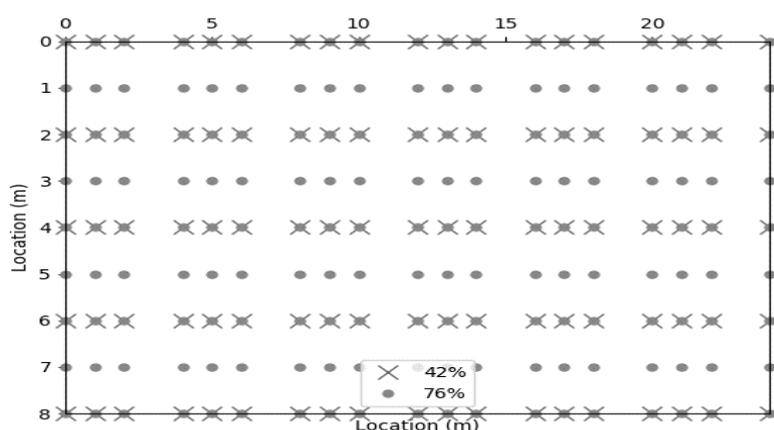
**Figure 3.** Reduced amount of fingerprint locations for RBF interpolated radio mappings estimation
