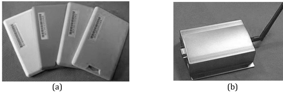
**Figure 1.** 2.4GHz RFID hardware used (a) RFID tags (b) RFID receivers
