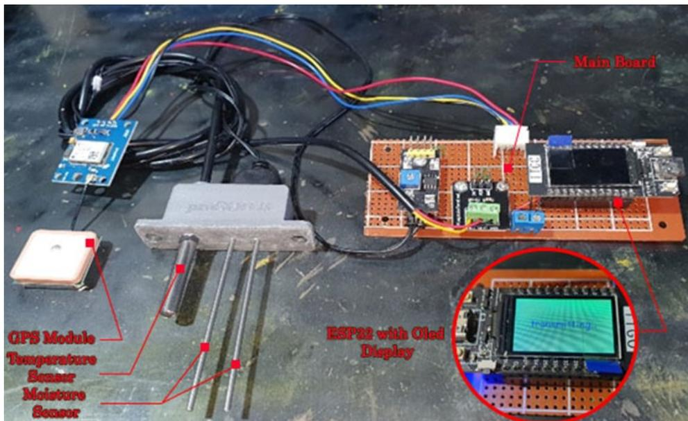
Figure 3. The Embedded Controller
