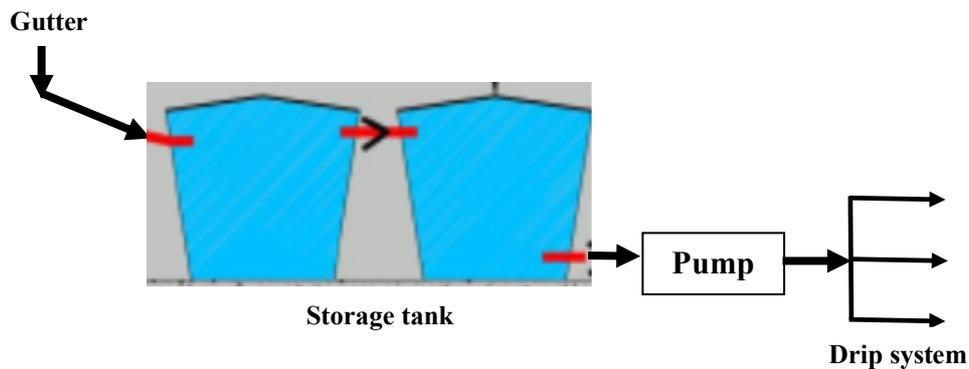
Figure 2. The developed irrigation system
