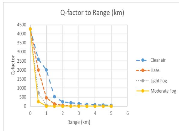
**Figure 8.** Q-factor to Range of WDM-MIMO FSO under different atmospheric conditions
