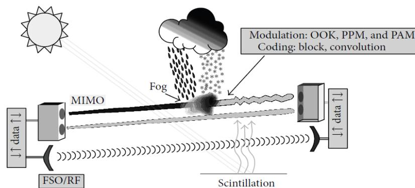
**Figure 1.** Effects of the atmosphere on the FSO system [7]
