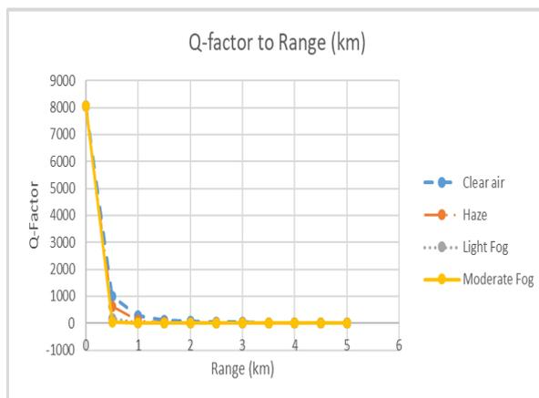
**Figure 7.** Q-factor to Range plot of SISO under different atmospheric conditions
