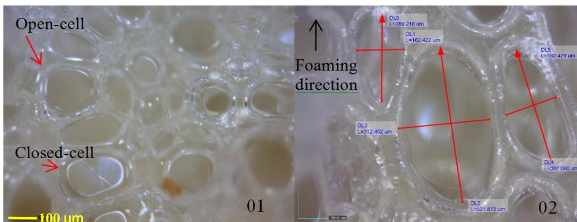
**Figure 1.** Micrographs of the reference sample from perpendicular (01) and parallel (02) to the foaming direction.
