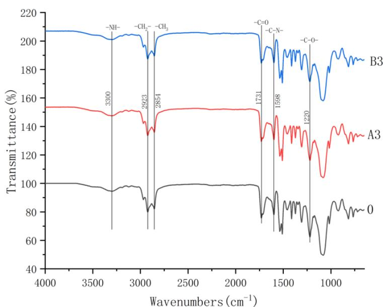
**Figure 3.** FTIR spectra of PU foam samples (0, A3, B3).
