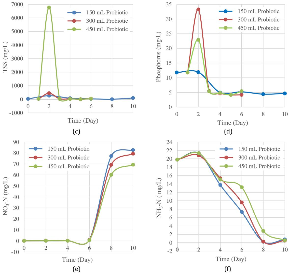
**Figure 2.** Performance of bench-scale probiotic batch treatment system for sewage treatment (a) COD (b) BOD (c) TSS (d) phosphorus (e)  $\text{NO}_3\text{-N}$ , and (f)  $\text{NH}_3\text{-N}$ .
