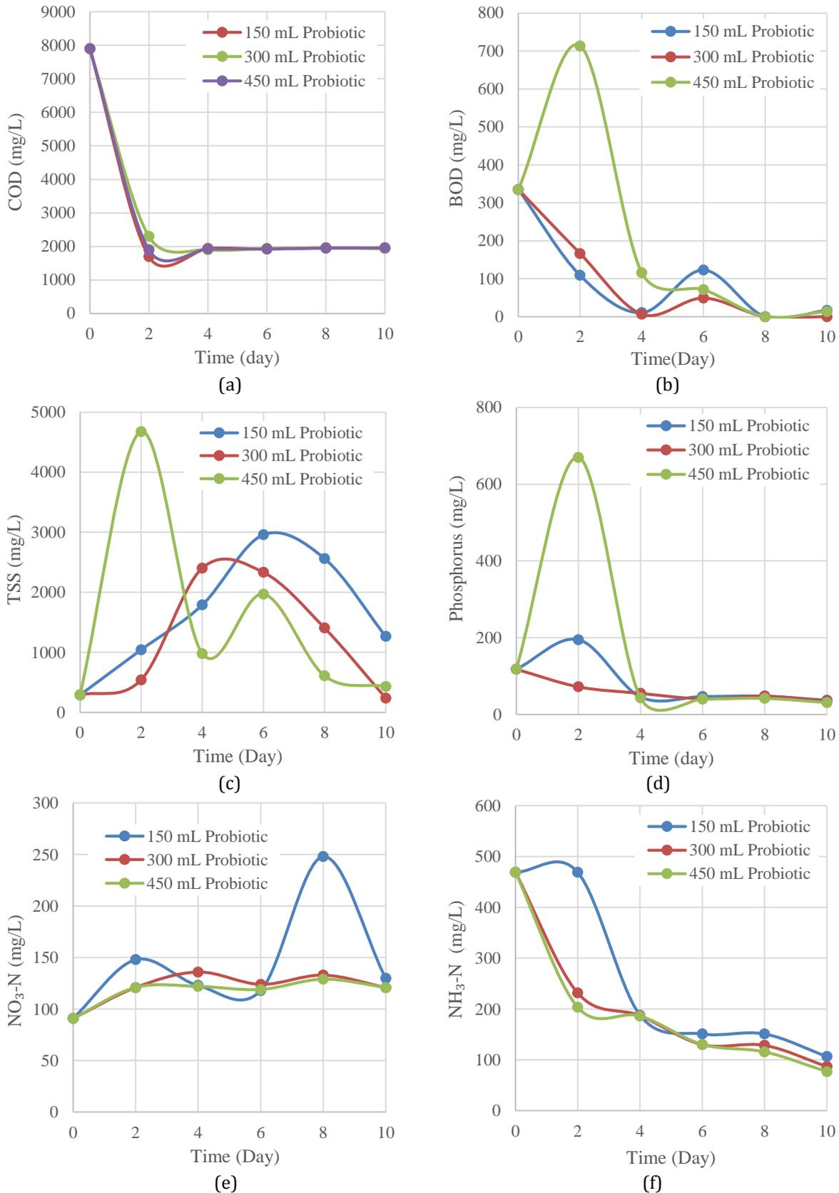
**Figure 3.** Performance of bench-scale probiotic batch treatment system for aerobic digested POME treatment (a) COD (b) BOD (c) TSS (d) phosphorus (e) NO<sub>3</sub>-N, and (f) NH<sub>3</sub>-N.
