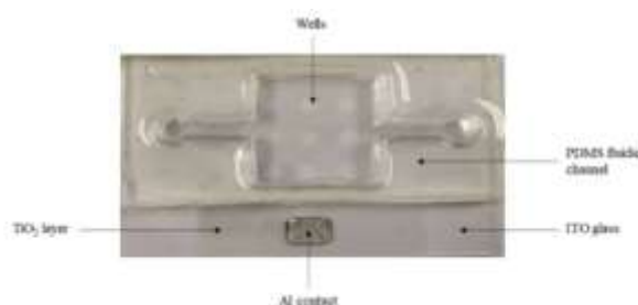
Figure 3. Top view of liquid-based memristor sensor.
