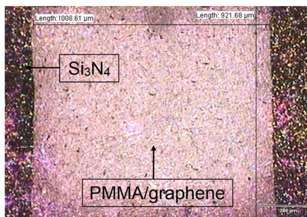
**Figure 5.** PMMA/Graphene membrane transferred by using 0.5 M FeCl<sub>3</sub>.
