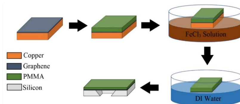
**Figure 2.** PMMA/Graphene film wet transferring process.
