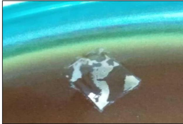
**Figure 3.** Etching process of CVD graphene using  $\text{FeCl}_3$  solution.
