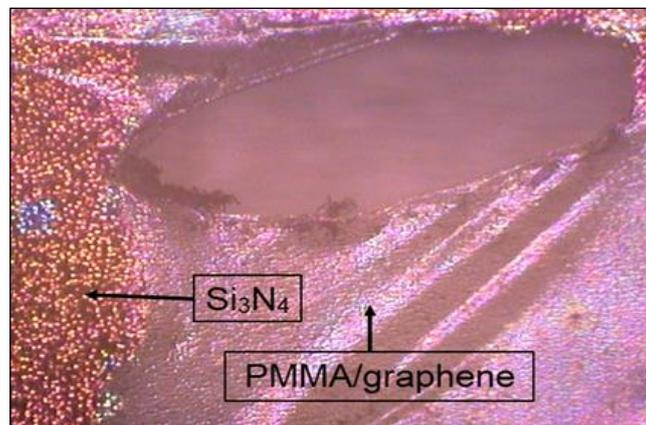
**Figure 7.** The tears of PMMA/Graphene membrane transferred by using 1.0M FeCl<sub>3</sub>.
