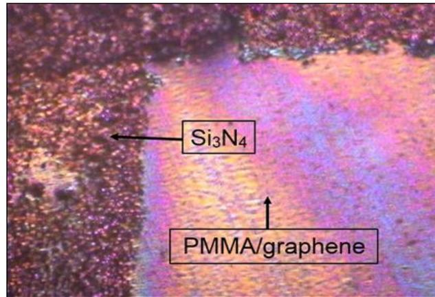
**Figure 6.** Close up image of PMMA/Graphene membrane transferred by using 0.5 M FeCl<sub>3</sub>.
