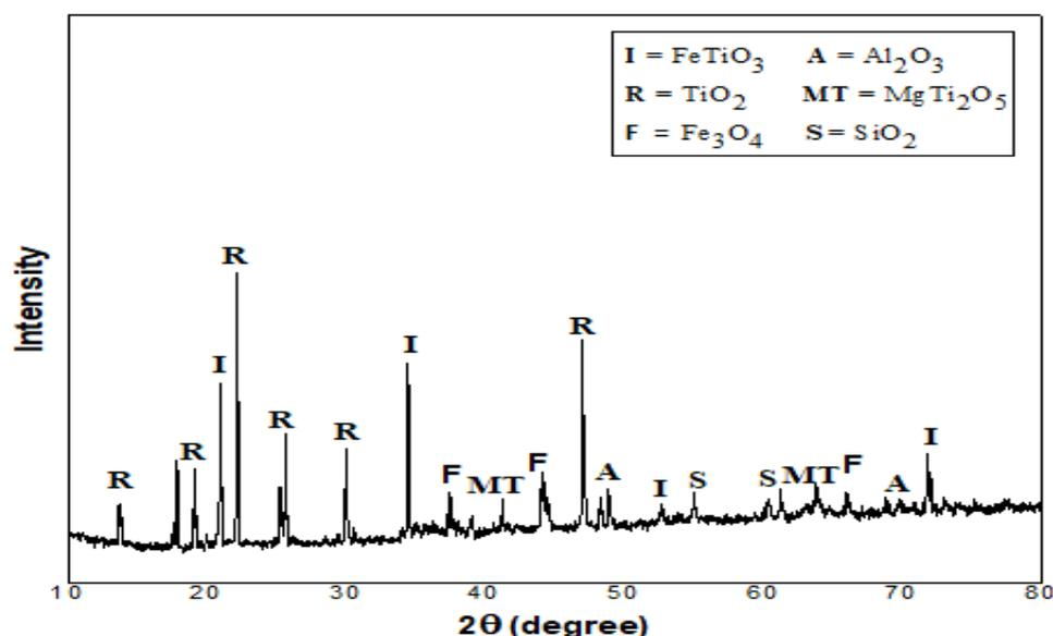
Figure 1. X-ray diffraction pattern of Langkawi ilmenite
