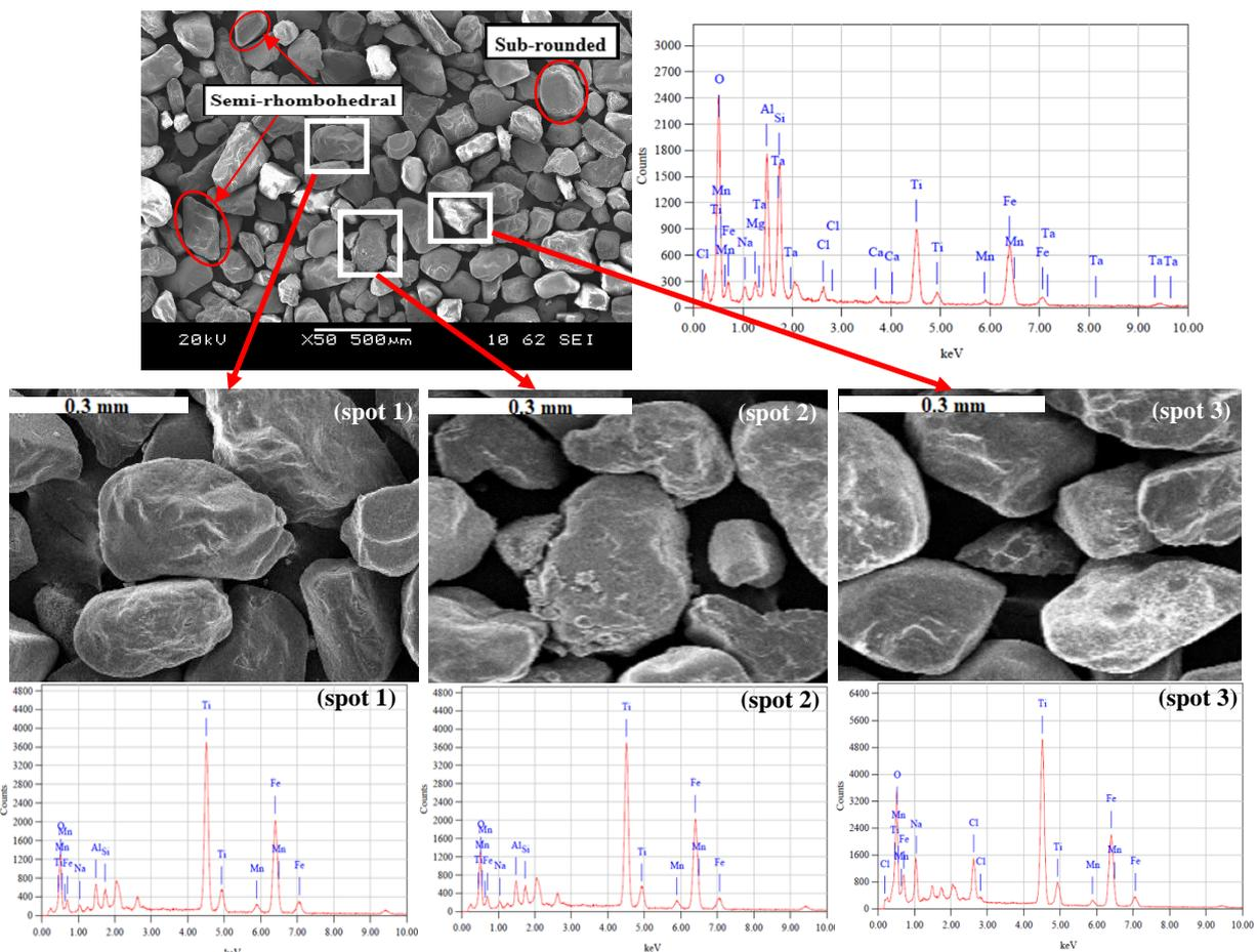
**Figure 2.** SEM/EDS images of Langkawi ilmenite ore and SEM/EDS analysis of specific rutile particle (spot 1), sub-rounded particle (spot 2) and semi-rhombohedral particle (spot 3)
