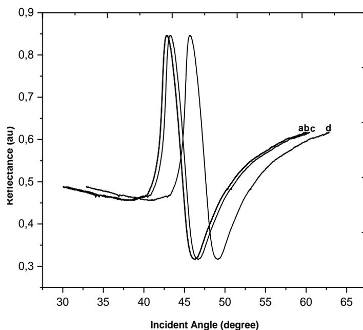
**Figure 5.** The SPR spectra of (a) Prism/Au (b) Prism/Au/Ag NPs (c) Prism/Au/Fe<sub>3</sub>O<sub>4</sub> NPs, (d) Prism/Au/Fe<sub>3</sub>O<sub>4</sub>@Ag NPs
