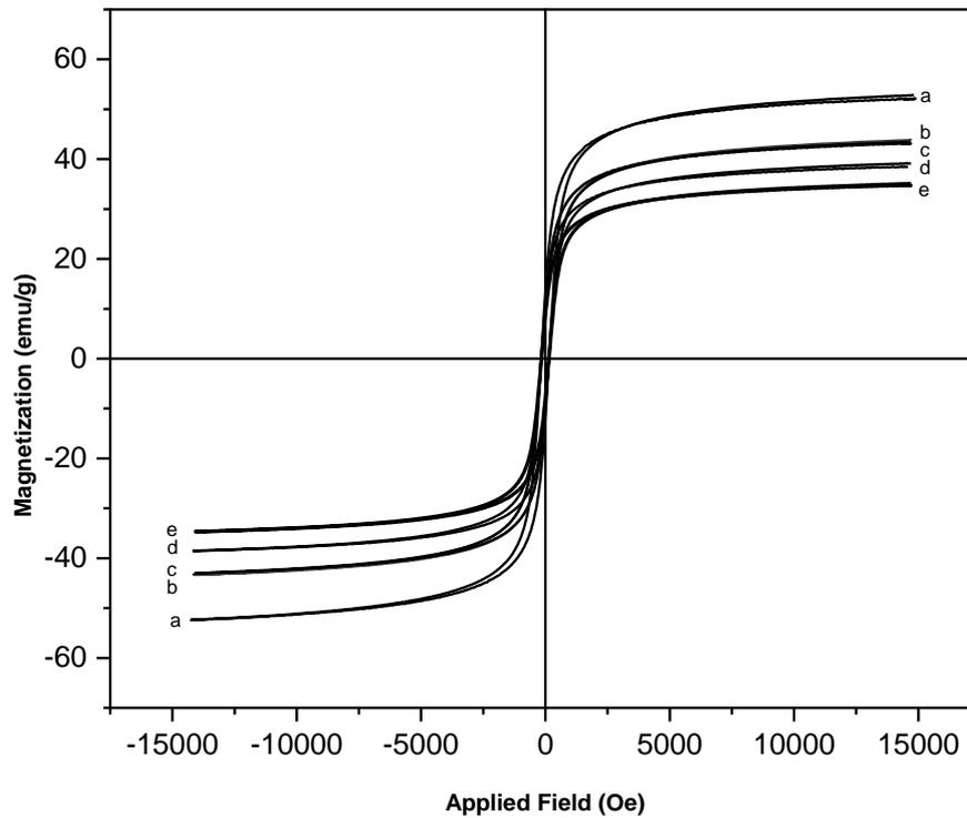
**Figure 3.** Magnetization versus applied magnetic field of core-shell  $\text{Fe}_3\text{O}_4@Ag$  NPs with various Ag concentration of (a) 20, (b) 40, (c) 60 (d) 80, and (e) 100 mM
