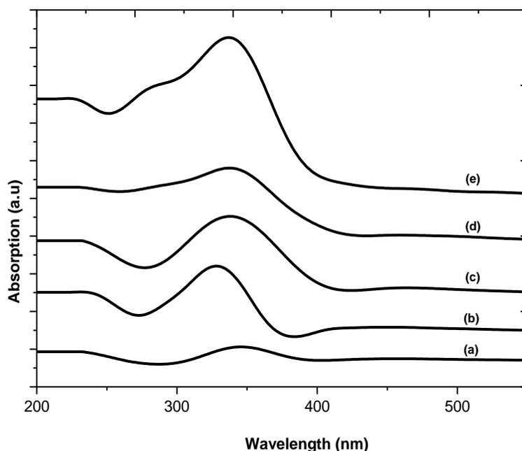
**Figure 4.** Spectrum of UV-Vis absorption of core-shell  $\text{Fe}_3\text{O}_4@Ag$  NPs with various Ag concentration of (a) 20, (b) 40, (c) 60 (d) 80, and (e) 100 mM
