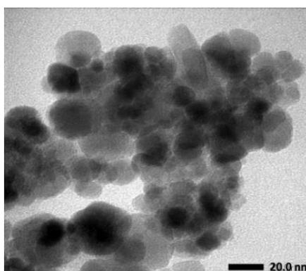
**Figure 2.** The TEM image of  $\text{Fe}_3\text{O}_4@Ag$  NPs 40 mM
