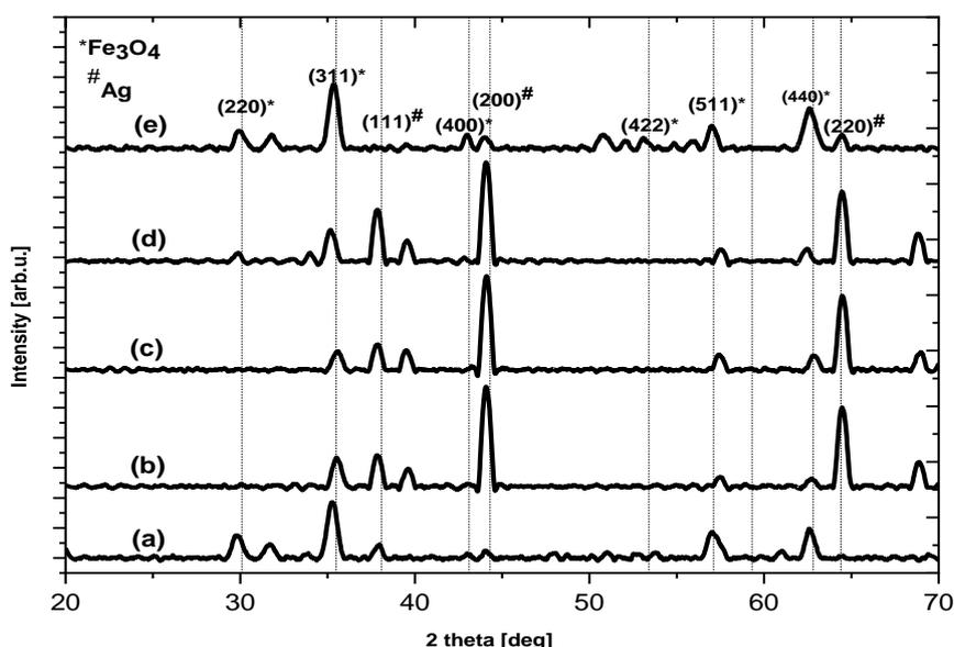
**Figure 1.** X-Ray patterns of core-shell Fe<sub>3</sub>O<sub>4</sub>@Ag NPs with various Ag concentration of (a) 20, (b) 40, (c) 60 (d) 80, and (e) 100 mM
