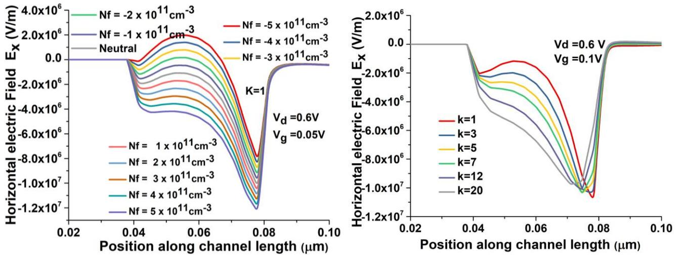
Fig 3. Electric field lines of SI\_NT\_TFET for various (a) dielectric constant ( $k$ ) and (b) charged biomolecule ( $N_f$ )
