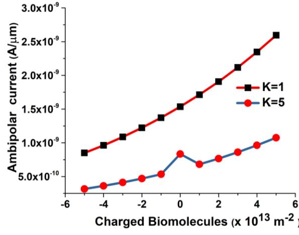
Fig. 4. Varying ambipolar current corresponding to charged biomolecules at k=1 and k=5
