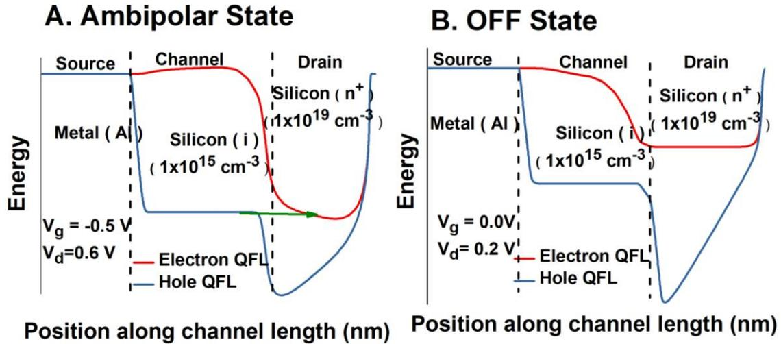
**Fig 2.** Quasi Fermi level for drain valance and channel conduction band at (a) ambipolar state and (b) OFF state
