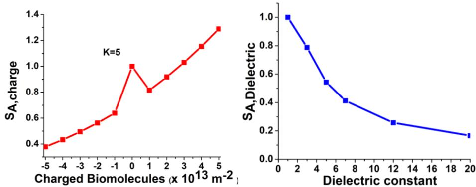
Fig. 5. Varying ambipolar sensitivity corresponding to (a) charged bio-molecules and (b) dielectric constant
