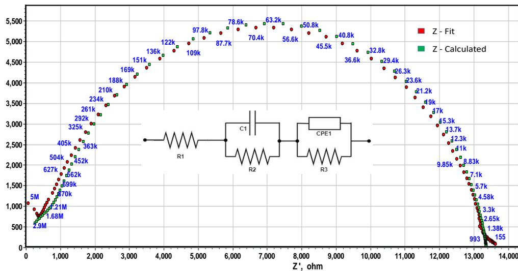
**Figure 3.** Complex plane Nyquist plot of HNO<sub>3</sub> doped polyaniline with its equivalent circuit
