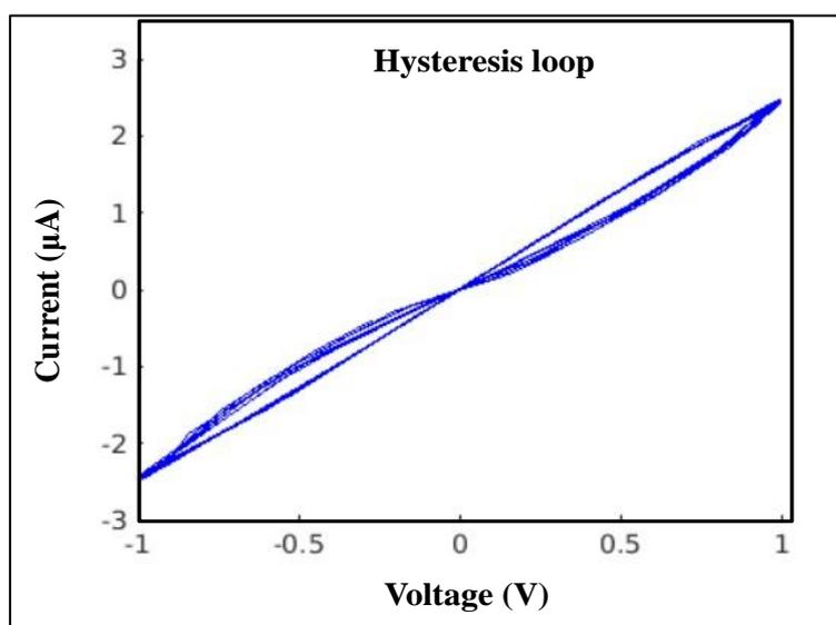
Figure 8. Hysteresis loop of the sensing element
