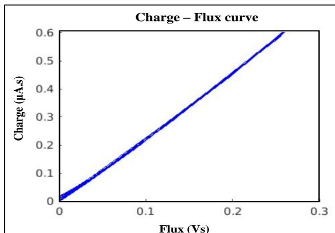
Figure 7. Charge-Flux curve of the sensing element
