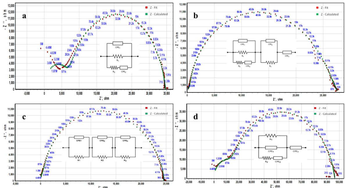
**Figure 4.** Complex plane Nyquist plot of polyaniline-WO<sub>3</sub> with its equivalent circuit: a) PANi - HNO<sub>3</sub> / WO<sub>3</sub> -5%, b) PANi - HNO<sub>3</sub> / WO<sub>3</sub> -10%, c) PANi - HNO<sub>3</sub> / WO<sub>3</sub> -15%, d) PANi - HNO<sub>3</sub> / WO<sub>3</sub> -20%
