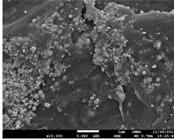
**Figure 5.** FESEM image of polyaniline-WO<sub>3</sub> nanocomposite with a doping concentration of 15%
