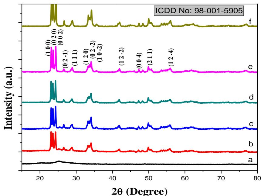
**Figure 2.** XRD patterns of: a) HNO<sub>3</sub> acid protonated PANi, b) PANi - HNO<sub>3</sub> / WO<sub>3</sub> -5%, c) PANi - HNO<sub>3</sub> / WO<sub>3</sub> -10%, d) PANi - HNO<sub>3</sub>/ WO<sub>3</sub> -15%, e) PANi - HNO<sub>3</sub> / WO<sub>3</sub> -20%, f) WO<sub>3</sub> nanoparticles
