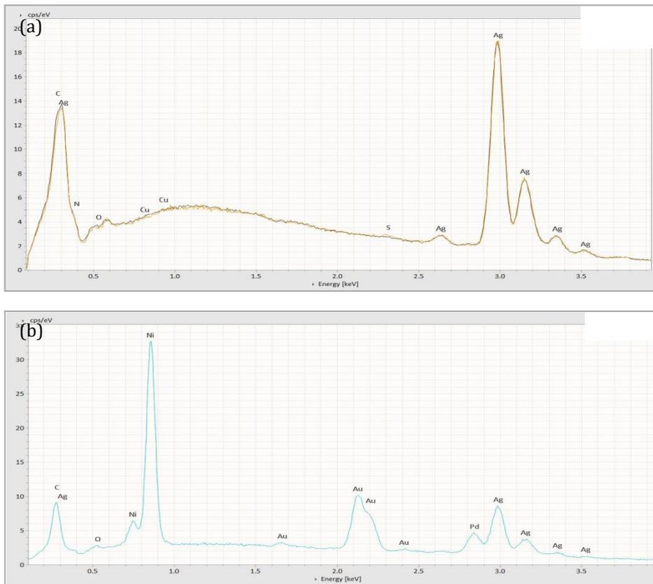
**Figure 5.** EDS spectra of; (a) standard Cu LF; (b) textured PPF.
