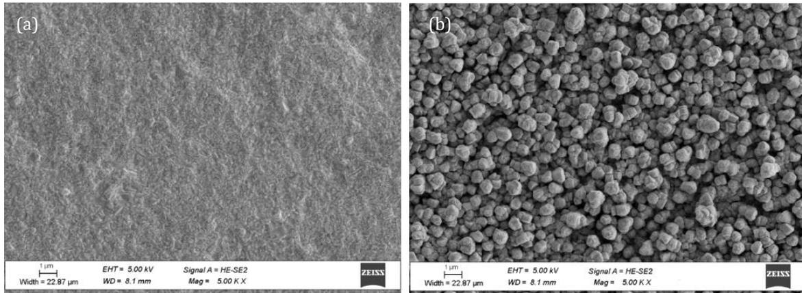
**Figure 4.** FESEM image of leadframe surface; (a) standard Cu LF; (b) textured PPF.
