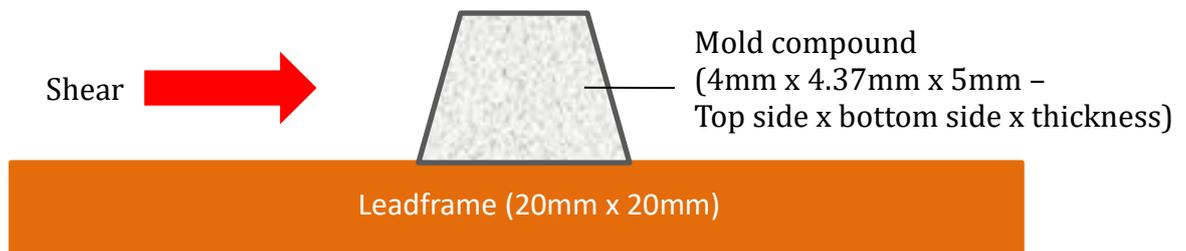
**Figure 2.** Schematic diagram of sample for mold shear strength test.
