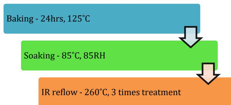
**Figure 3.** Process flow for pre-conditioning MSL level 1.
