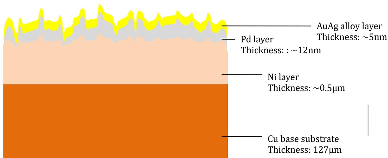
**Figure 1.** Configuration of metal layer plating and surface texturing for PPF.
