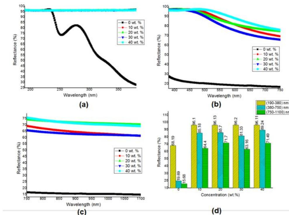
**Figure 5.** UV-VIS reflectance spectra of PVA/molasses composite at different concentrations of molasses (0, 10, 20, 30 and 40 wt.%)
