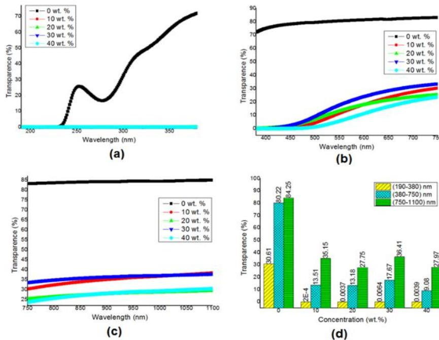
**Figure 4.** UV-VIS transparency spectra of PVA/molasses composite at different concentrations of molasses (0, 10, 20, 30 and 40 wt.%)
