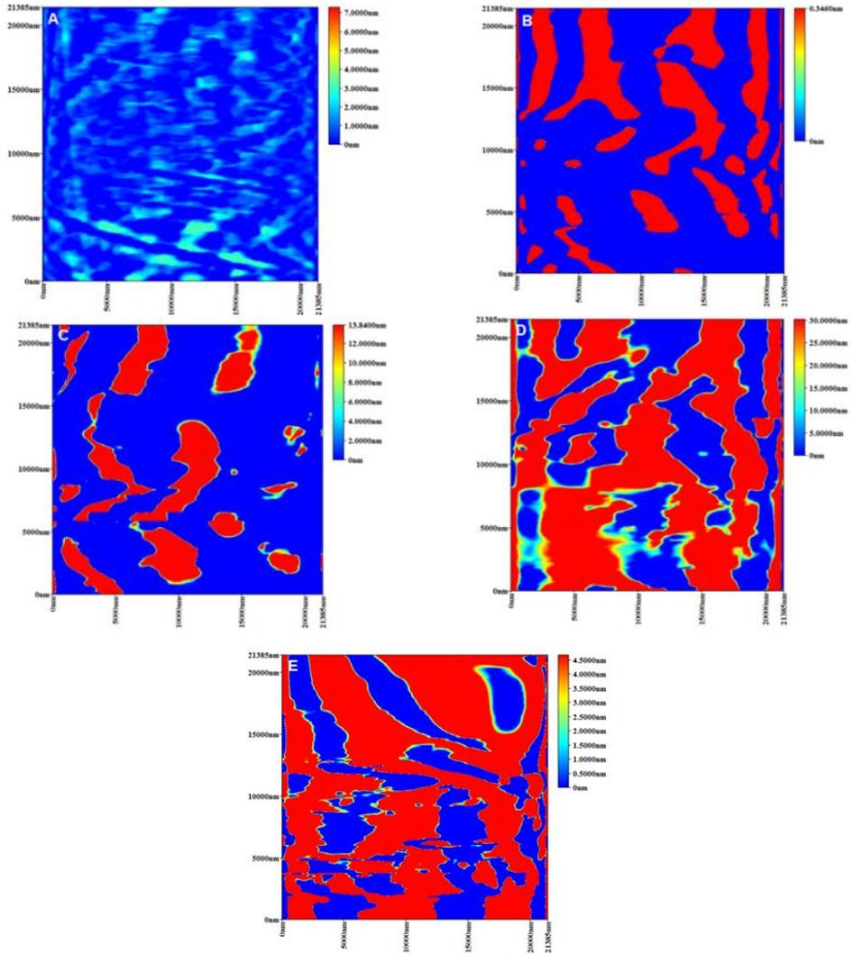
**Figure 6.** AFM 2D topography images of PVA/molasses composite at different concentrations of molasses (0, 10, 20, 30 and 40 wt.%)
