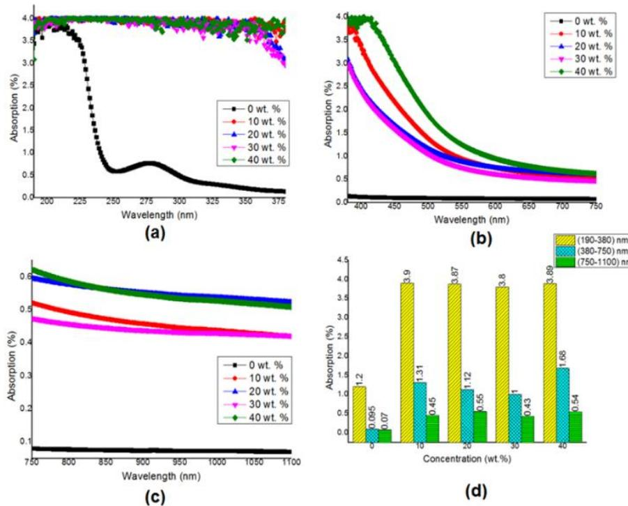
**Figure 3.** UV-VIS absorption spectra of PVA/molasses composite at different concentrations of molasses (0, 10, 20, 30 and 40 wt. %)
