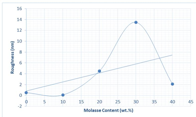
**Figure 7.** Roughness average curve of PVA/molasses composite surface by AFM at different concentrations of molasses (0, 10, 20, 30 and 40 wt.%)
