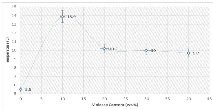
**Figure 11.** Difference maximum temperatures curve between before and after demonstration of sun light for 1 minute of PVA/molasses composite by IR camera at different concentrations of molasses (0, 10, 20, 30 and 40 wt.%)
