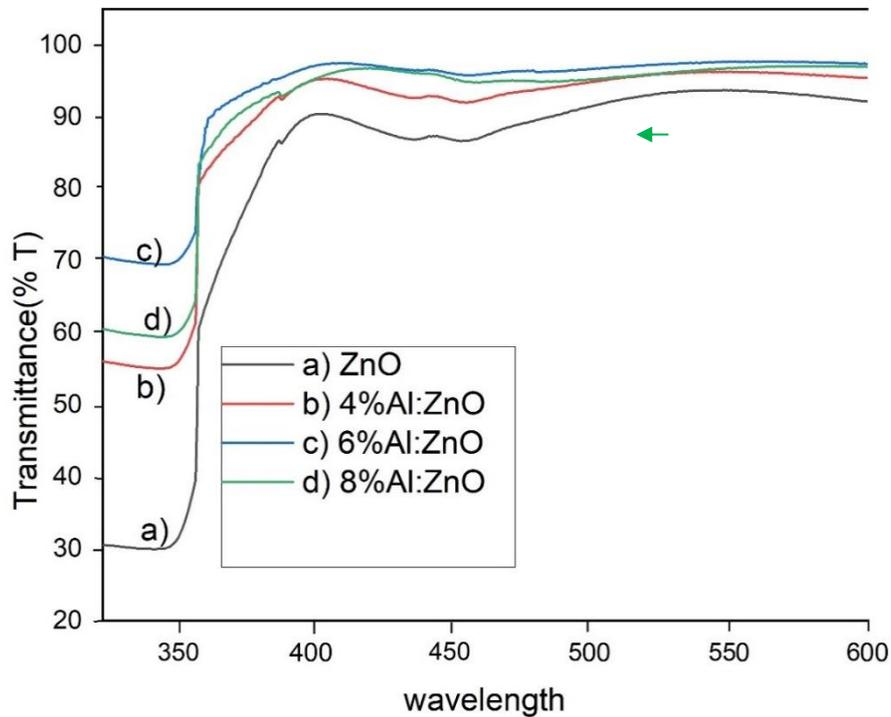
Fig. 5: Transmittance spectra of the undoped and Al doped ZnO thin films. The inset zoom image magnifies the blueshift of absorption edge
