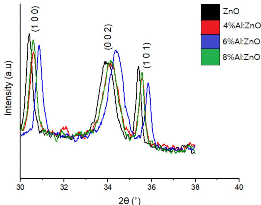
Fig. 1: XRD pattern (zoom) of the preferred peaks showing a clear shifting towards higher angle
