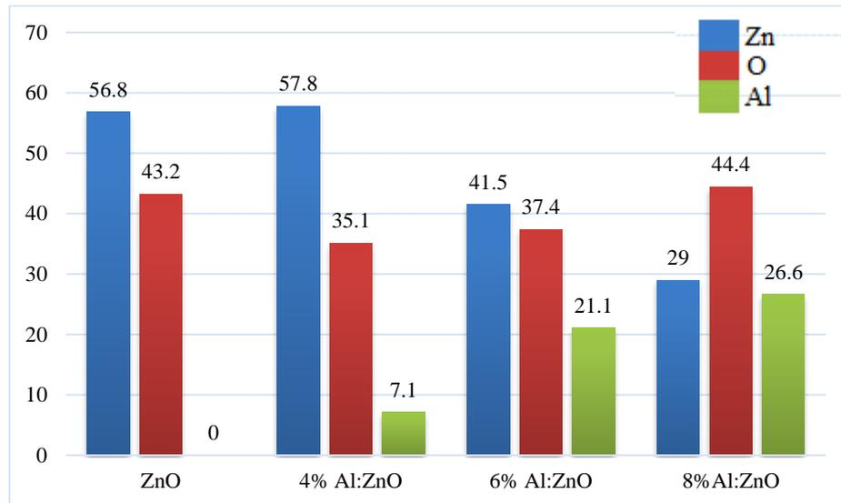
Fig. 4: Elemental compositions of the thin films by EDS analysis
