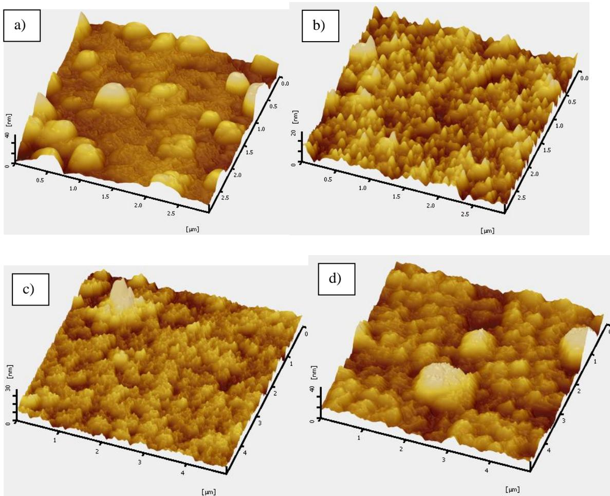
Fig. 3: AFM surface topography of undoped and Al-doped ZnO thin films
