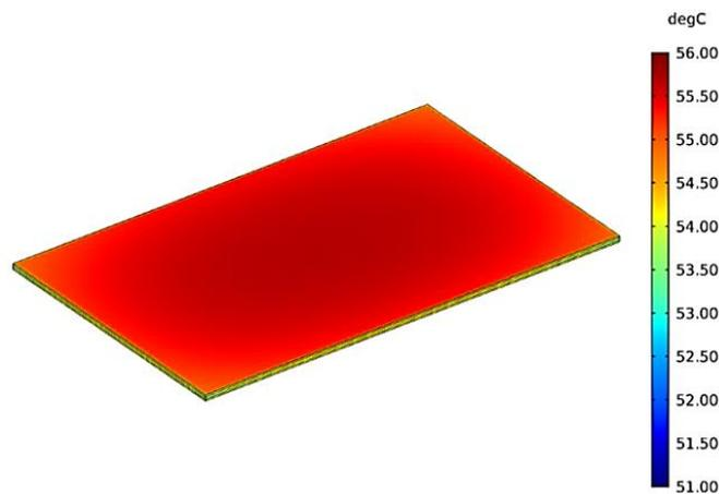
**Figure 2.** Temperature distribution in the photovoltaic cell structure without cooling ( $^{\circ}\text{C}$ )
