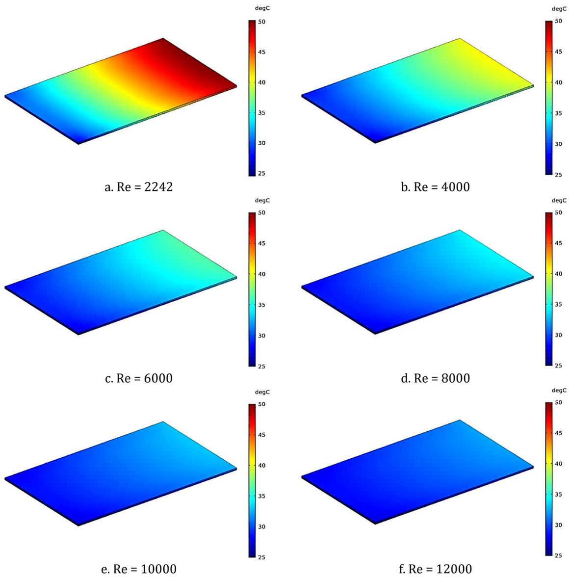
**Figure 3.** Temperature distribution in the photovoltaic cell structure with water cooling ( $^{\circ}\text{C}$ ) for a range of Reynolds numbers
